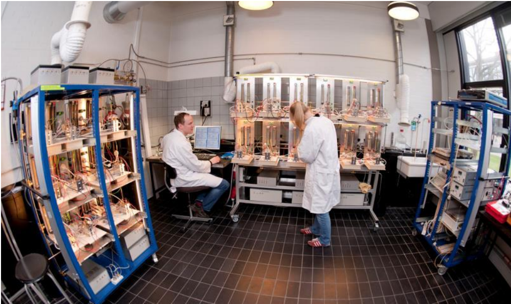
Fig, 24 24 cells durability test setup, for long term testing
