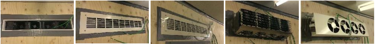
Figure 3: Pictures of the different configurations tested (from left to right: no grille / grille / grille with cover / mixer 1 / mixer 2).
