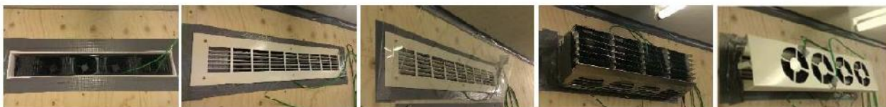
Figure 3: Pictures of the different configurations tested (from left to right: no grille / grille / grille with cover / mixer 1 / mixer 2).
