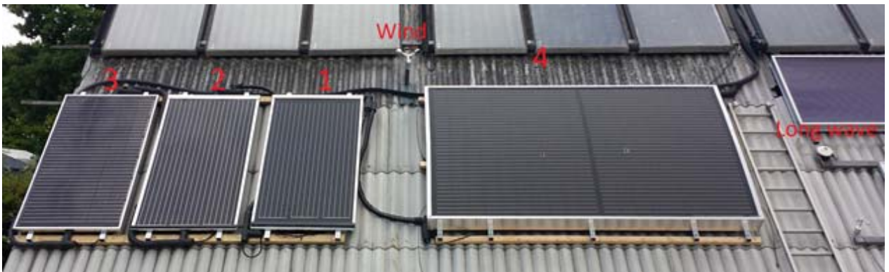
Figure 1. The prototype collectors tested. They are connected in series and have the same flow rate. The collector size is 2 m 2 respective 6 m 2 .
