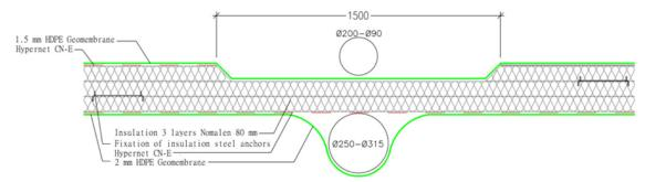
Fig. 6: Cross section of the weight pipes on the floating liner.
