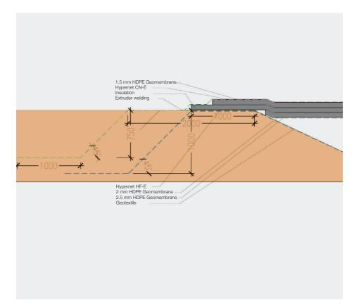
water from Dronninglund water company was used, but oxygen salts and calcium were removed from the water. The lid is constructed by welding a 2 mm polyethylene liner onshore and pulling it gradually over the water. Thereafter, the insulation is constructed on top of the liner, floating on the water.
