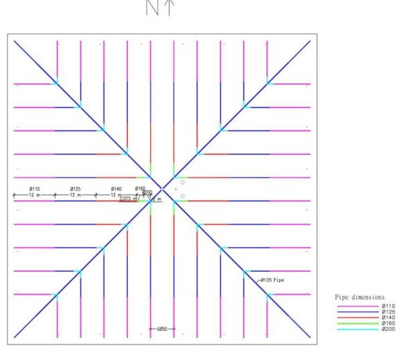
Fig. 8: Weight pipe layout on the top of the cover.
