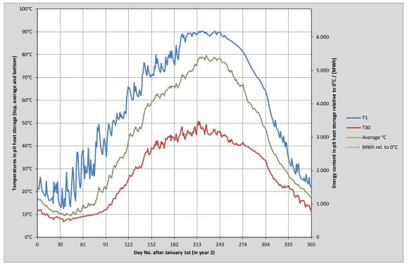
Fig. 9: Calculated temperatures in the pit heat storage year 2.
