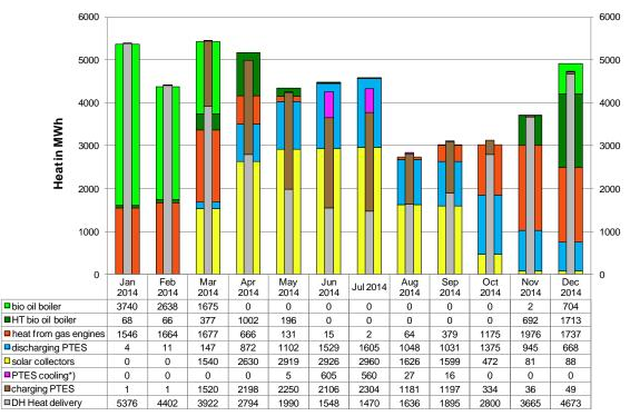
*Fig.* **18**: Monthly system heat balance according to 2014 monitoring data. \*) Night cooling of PTES by way of solar collectors because of high temperatures.
