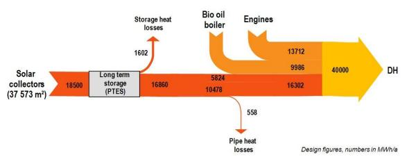
Fig. 16: Yearly energy flow diagram according to design figures, see Table 2.
