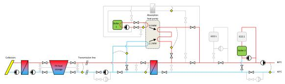
**Fig. 4:** Principle diagram, SUNSTORE 3. Yellow squares are flow/energy meters. The diagram is simplified and not all equipment is shown.
