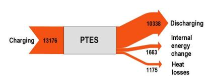
Monitoring results 2014, numbers in MWh/a **Fig. 20:** PTES heat balance according to 2014 monitoring data.
