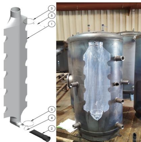
Figure 16: Double Sided Stratifier - Drawing and Installation at a customer
