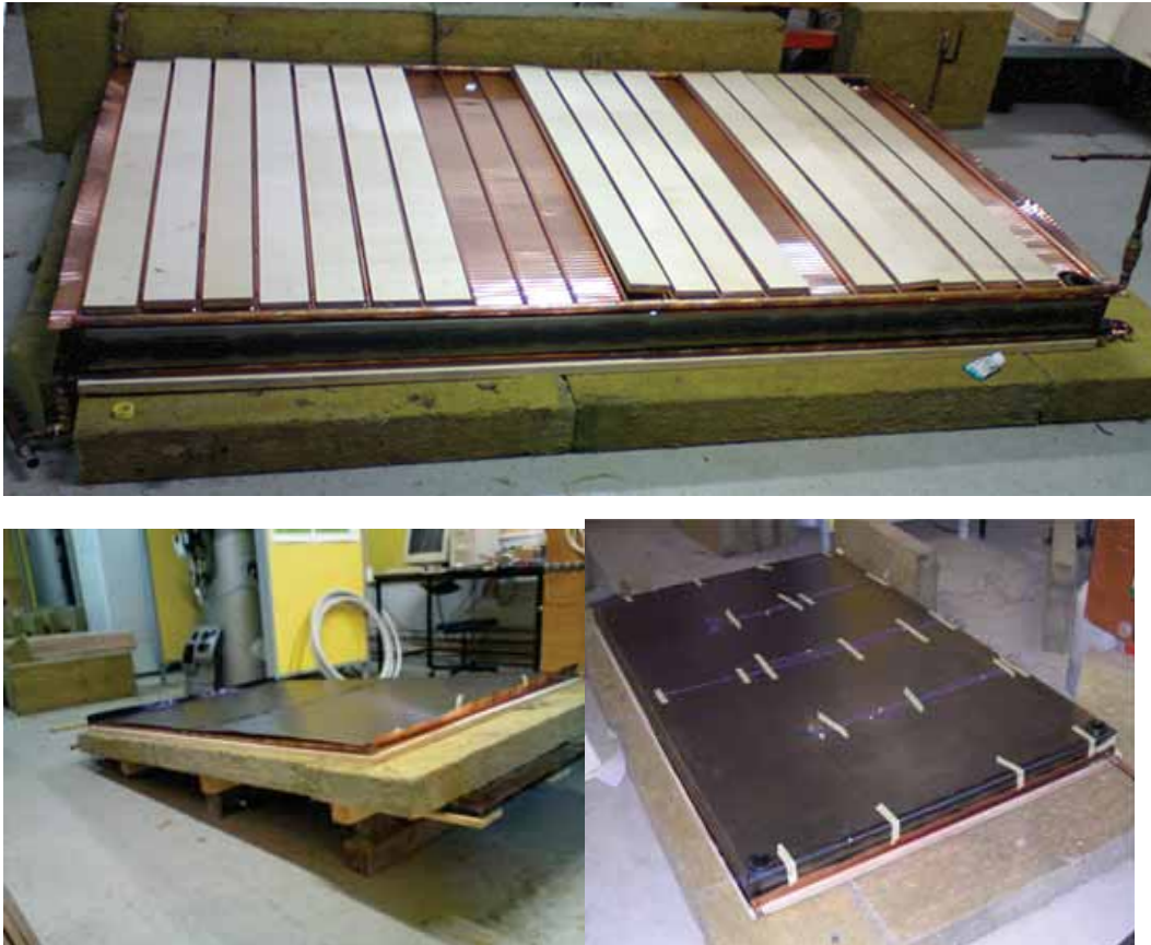
Figure 5: Photos of the first heat storage module.
