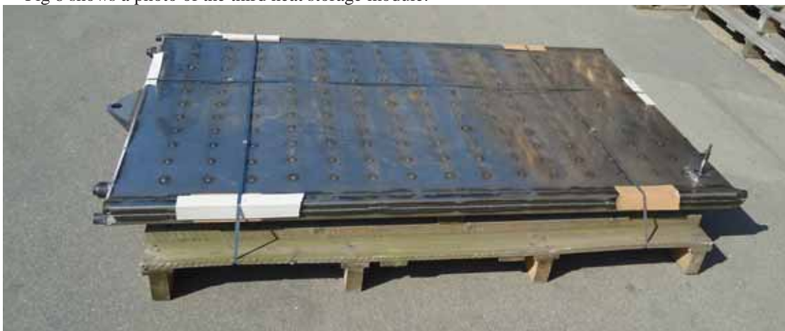
Fig. 8. Photos of the third heat storage module with two holes at the left hand side of the module used to fill in the salt water mixture.
