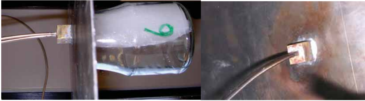
Fig. 4. Photos of the setup with cooling through a steel plate.
