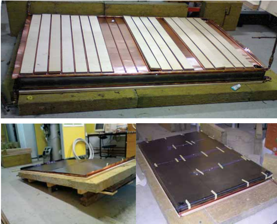
Fig. 3. Photos of the first heat storage module.
