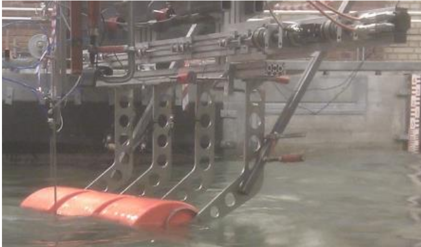
Figure 3: The PTO test model, where the new design of the PTO was tested and optimized.
