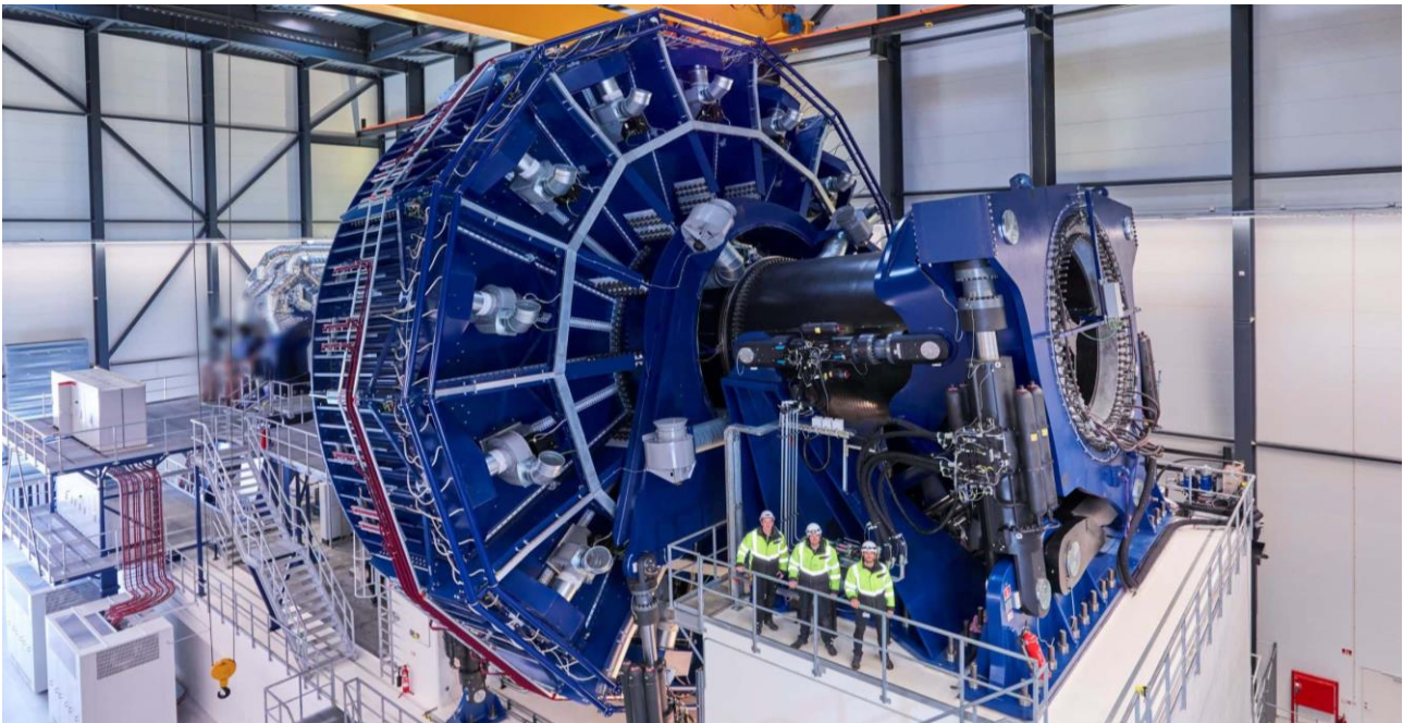
Figure 1-20: A picture of the 25MW HALT-XL nacelle test bench at LORC.
