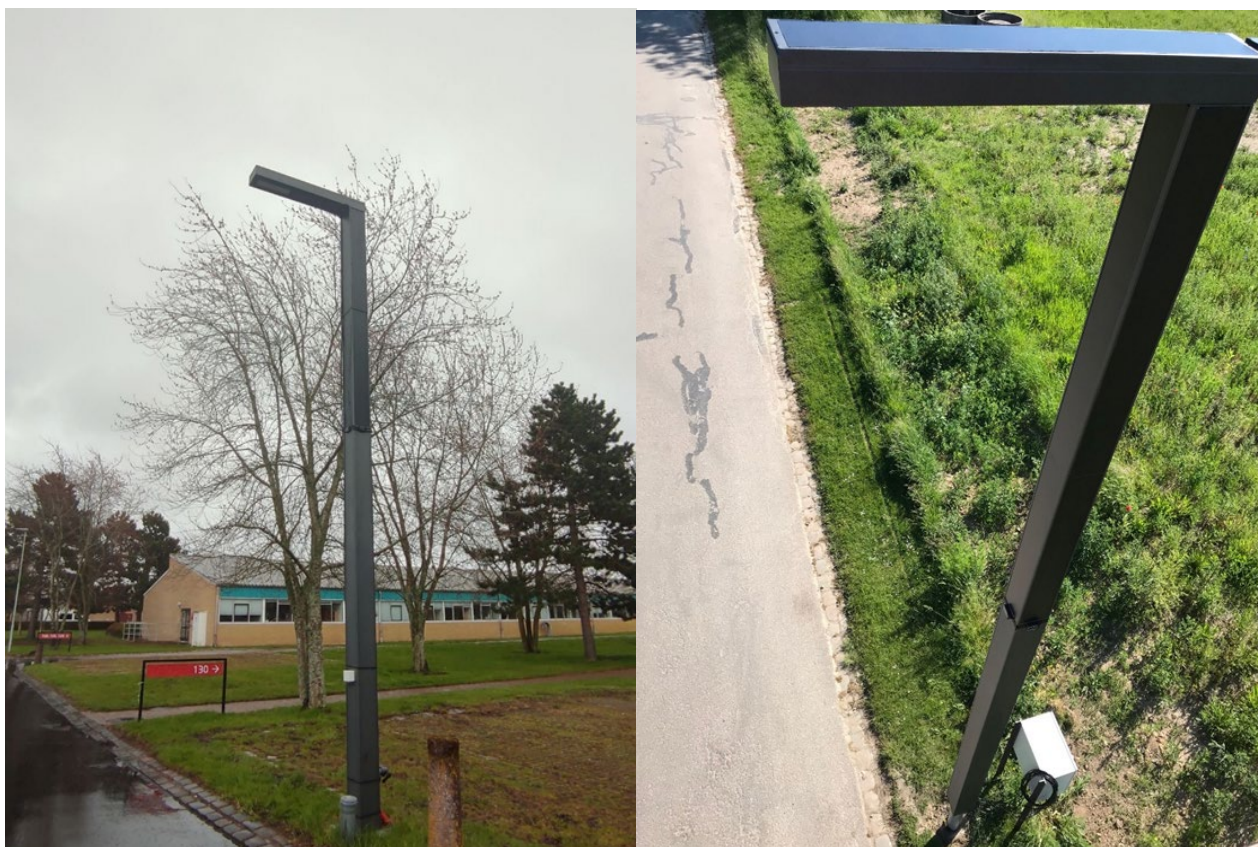
Figure 2 - Left: SolarDesign version 1 for baseline. Right: SolarDesign, version 2 with upgraded electronics, IoT and battery system.
