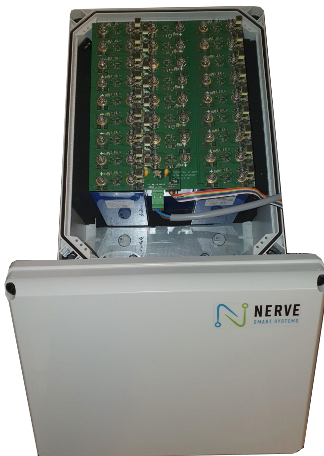
Figure 21 – EMS and battery system integrated in a box.
