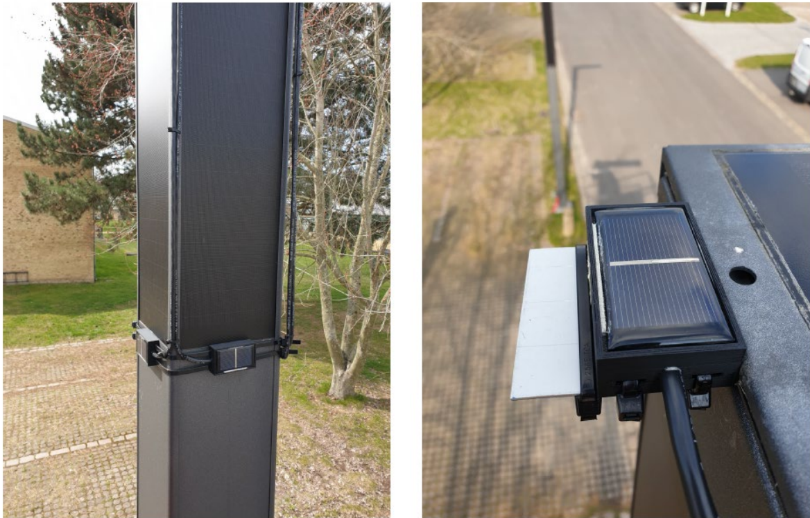
Figure 3 - Left: Irradiance sensors on sides. Right: Irradiance sensors on top.
