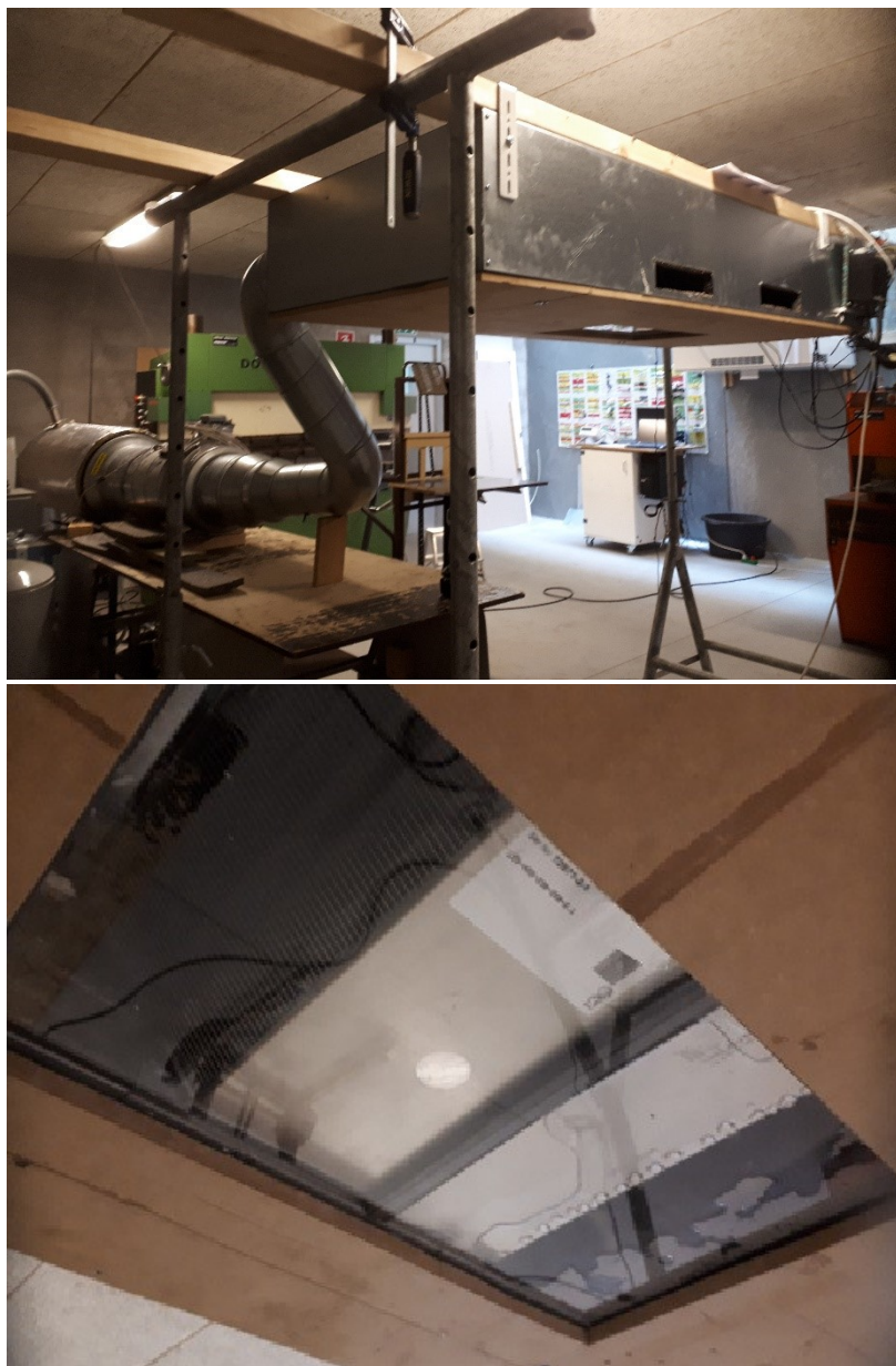
Figure 12: Early model experiment, observing two-way removal of condensate from counterflow heat exchanger through glass panel in bottom.
