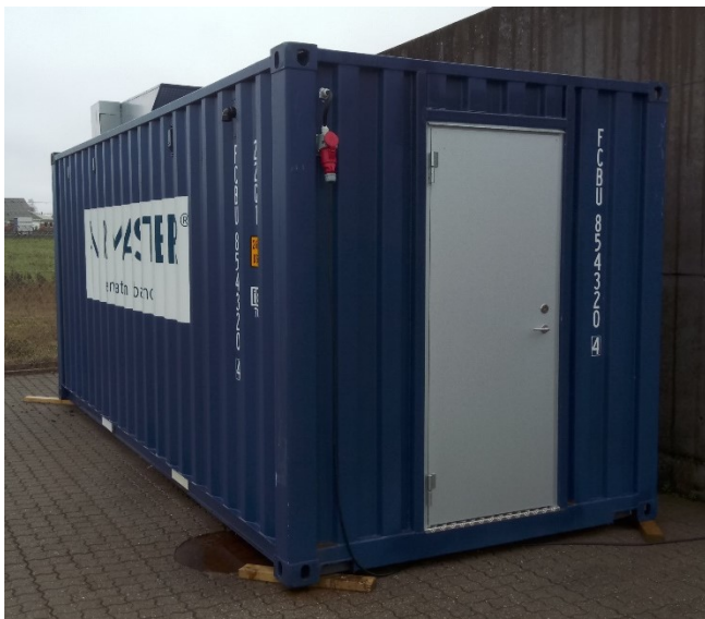
Figure 6: Climatic laboratory, built for COP/EER tests inside a container
