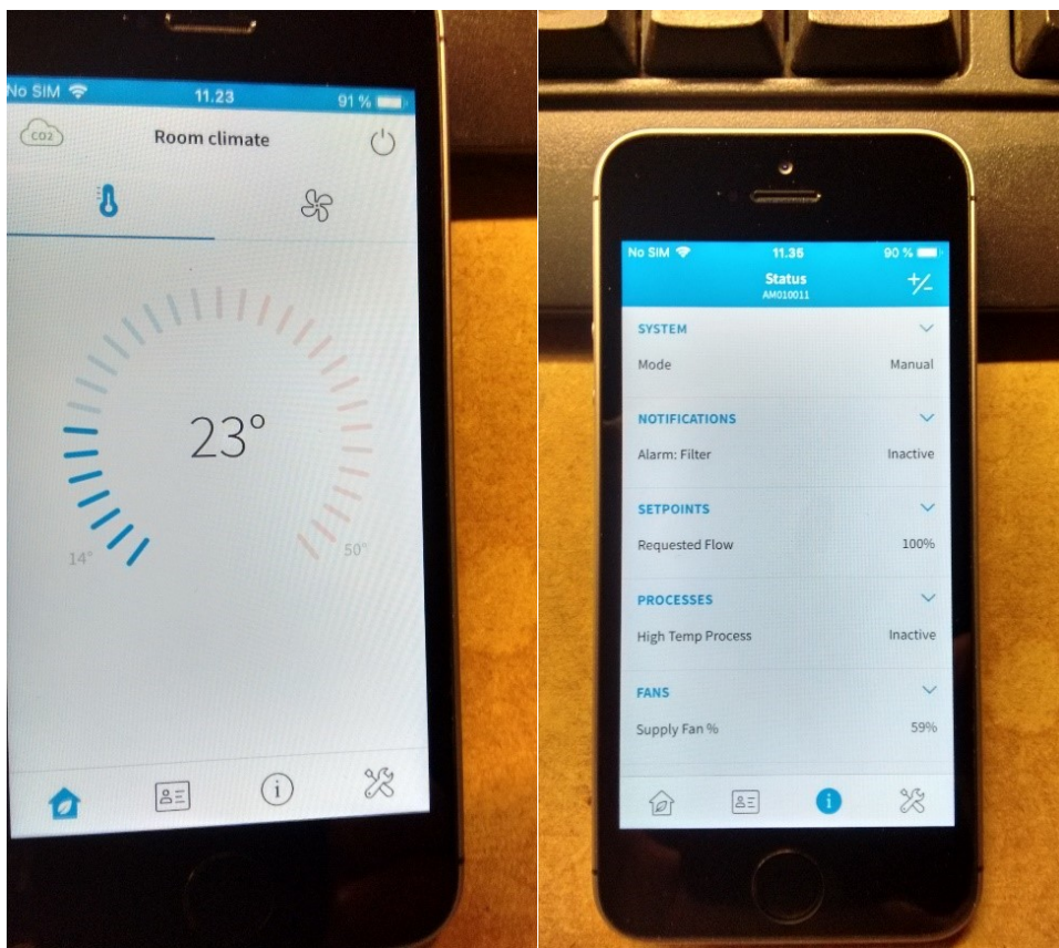
Figure 9: User interface by smartphone app. Left: easy to understand choices for modifying automatic settings, if wanted. Right: Status window, for the technically interested.
