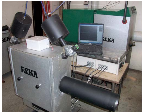
Figure 5: ESP for smaller wood pellet boiler. The filter is with two channels and rotating plate collectors with a diameter of 250 mm.
