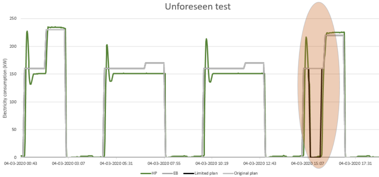
Figure 25: Data from the FlexHeat facility compared to the original plan and the unforeseen capacity limitation.
