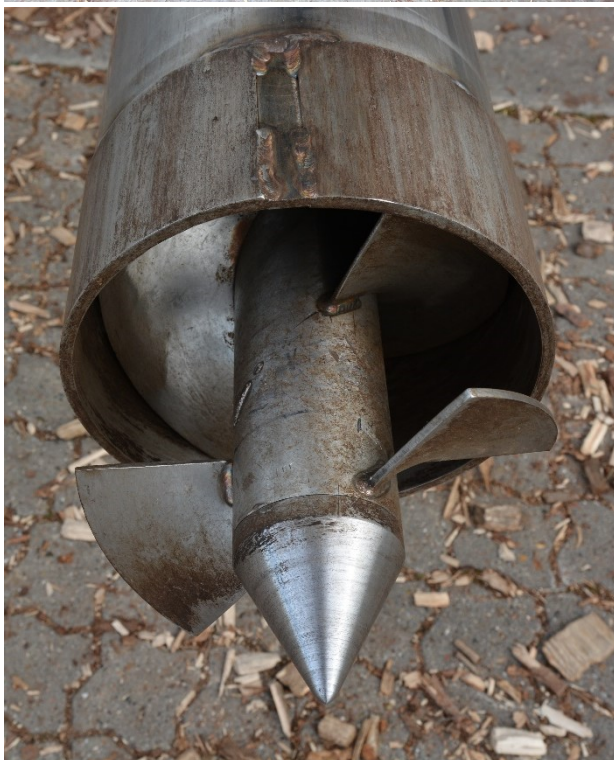
Figure 7: Test of the sampler/divider at Aabybro. Top left: sampler suspended above wood chip pile, top right: sampler lowered towards pile, bottom left: sample intake (detail), bottom right: samples are extracted at the top of the screw conveyor.
