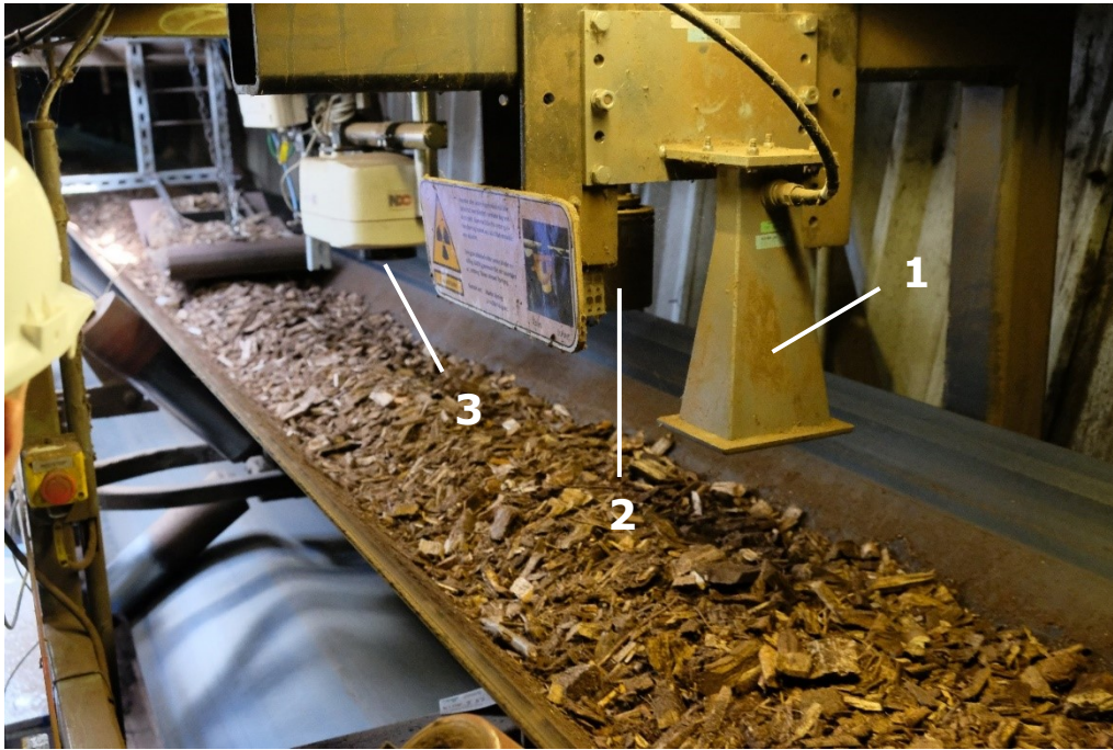
Figure 1: Microwave (1) and NIR (3) installed on the conveyor belt. The microwave instrument consists of a transmitter and a receiver, which are placed below (not visible in the image) and above the conveyor, respectively. The device for measuring area density to complement microwave measurements is the small black box to the right of the warning sign (2).
