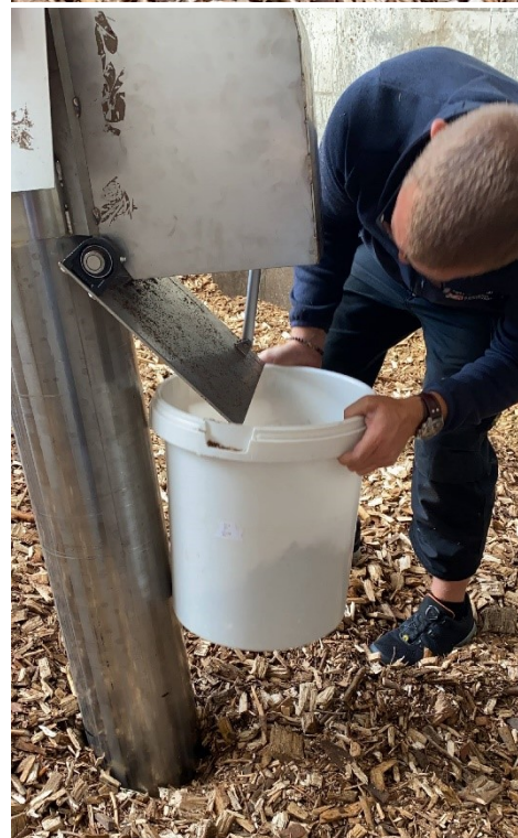
Figure 7: Test of the sampler/divider at Aabybro. Top left: sampler suspended above wood chip pile, top right: sampler lowered towards pile, bottom left: sample intake (detail), bottom right: samples are extracted at the top of the screw conveyor.
