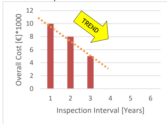
Figure 40: LEFT - A trend can be observed based on 3 analyzed maintenance strategies with different inspection intervals. According to the trend, increasing time intervals between inspection leads to a decrease in overall cost over the blade lifetime. RIGHT - The graph shows inspection interval vs overall cost. The optimal inspection interval has been found at the lowest point of the graph to be 4½ years. The trends suggest increasing or decreasing inspection intervals depending on the analyzed data and if it is for more or less than 4½ years inspection interval.
