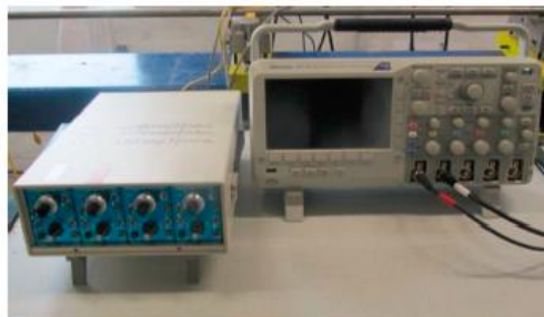
Figure 4.7 - Equipment used to record the strain gauge signals
