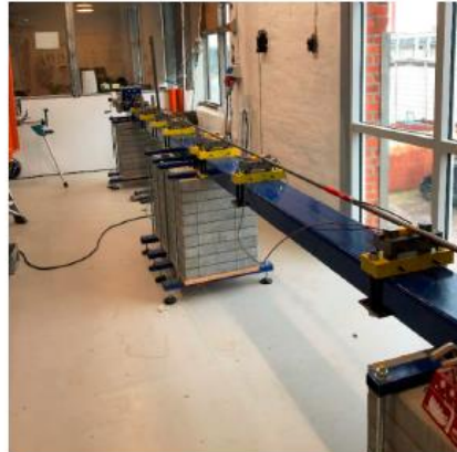
Figure 3-1 - Torsional split Hopkinson bar for high strain rate shear testing
