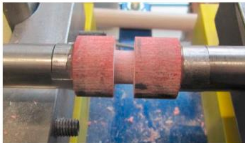
Figure 4.12 - Test sample bonded to end caps and mounted on the input and output bar spigots
