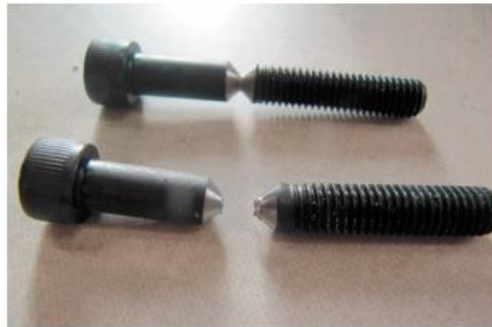
Figure 4.4 - Snap bolts used to tighten the clamp shoes
