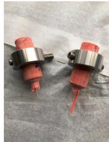
Figure 2-4 – Fractured test sample
