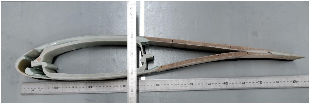
Figure 0.22 - Blade cross section 1 meter from tip
