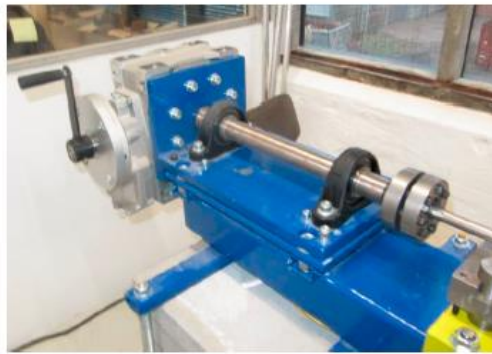
Figure 4.2 - Torque head used to twist the clamped section of the input bar
