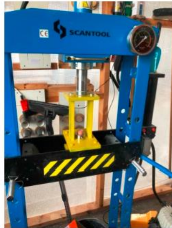
Figure 2-3 – Test sample mounted in hydraulic press
