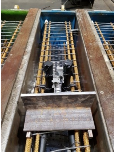
Figure 12: a) Single-U pipe attached to the steel reinforcement cage. b) Energy pile cross section. Dimensions are given in cm.
