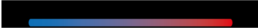
Figure 33: Geothermal pipe in the ground of length L with inlet and outlet temperature T_{f,i} and T_{f,o} , respectively. In this illustration, the pipe absorbs heat from the ground, elevating temperature at the outlet.
