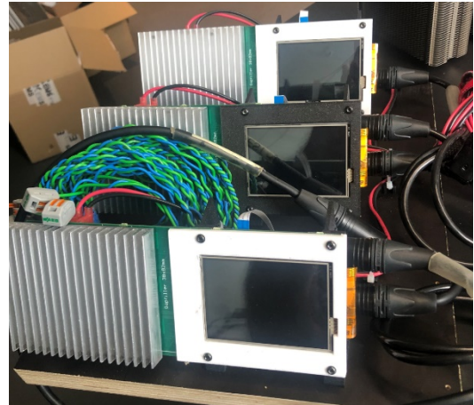
Figure 10. Left: schematic of the laser power supply system to set the current of the six laser diode arrays. Right: photo of the three driver boards with touch screen control.
