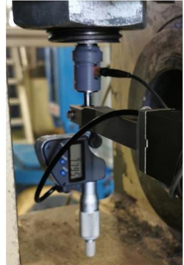
The threaded rod is positioned on the tension machine, and the nuts are tightened by hand. The clamping length, including washers are measured by a measuring tape, to be able to calculate the pretension of the bolt, based on the elongation.
