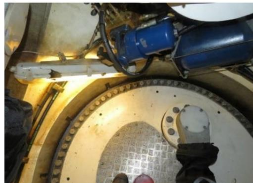
Consist of yaw-ring, bearing, brake-grips, brake-pads and all relevant bolts according to different system designs. No major problems are noticed. However, in general more focus is needed on wear and tear on the brake-pads.
