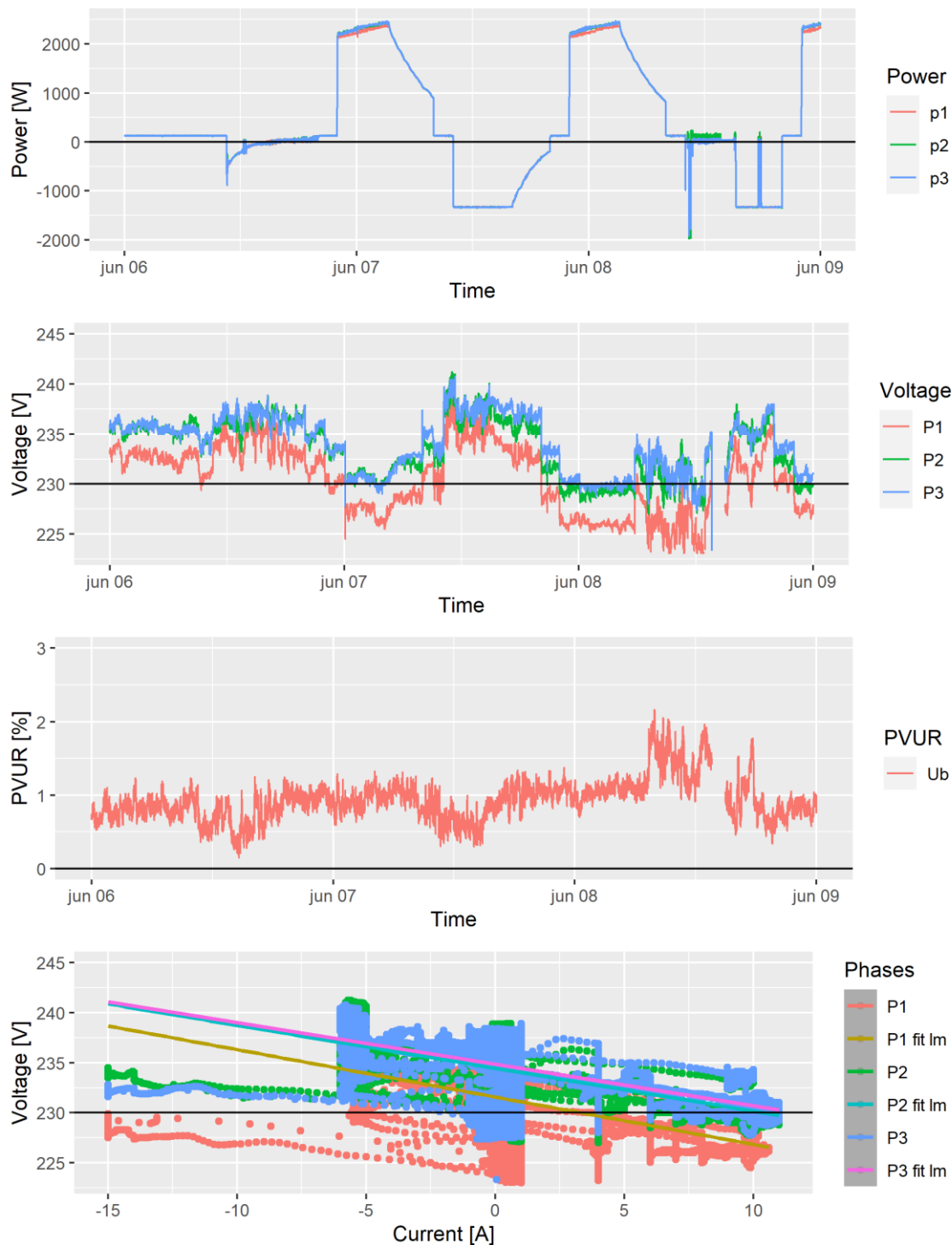
Figure 4 a) Power of battery 2, charge and discharge circles. b) Phase voltages for battery 2. c) PVUR for the duration of test 1. Power of battery 2, charge and discharge circles. d) Voltage ~ Current plot for all three phases with fitted values.
