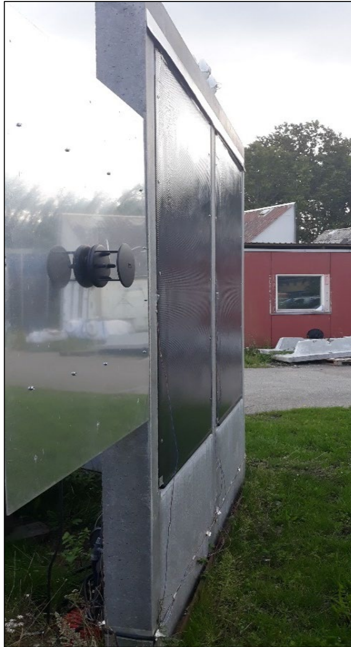
Figure 23. Location of the ultrasonic wind sensor.
