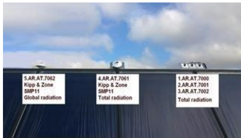
Fig.3. The pyranometers in the middle of the flat plate collector field [29]
