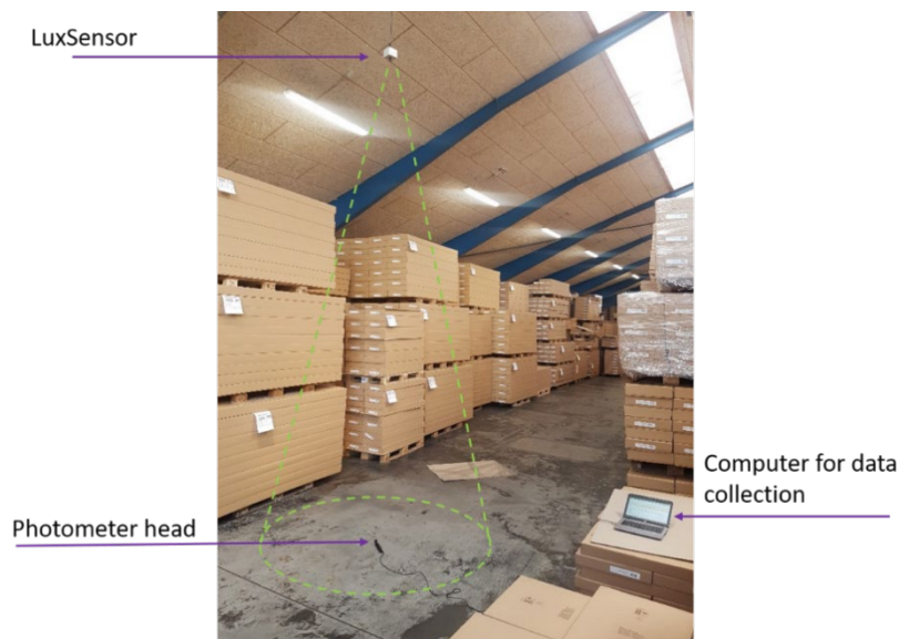
Figure 8. Photo of on-site calibration where the field of view of the luxsensor is indicated by the green dashed cone, the reference photometer is connected to the computer and measured over time.
