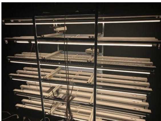
Figure 14. Photo of the long term test setup for LED tubes.
