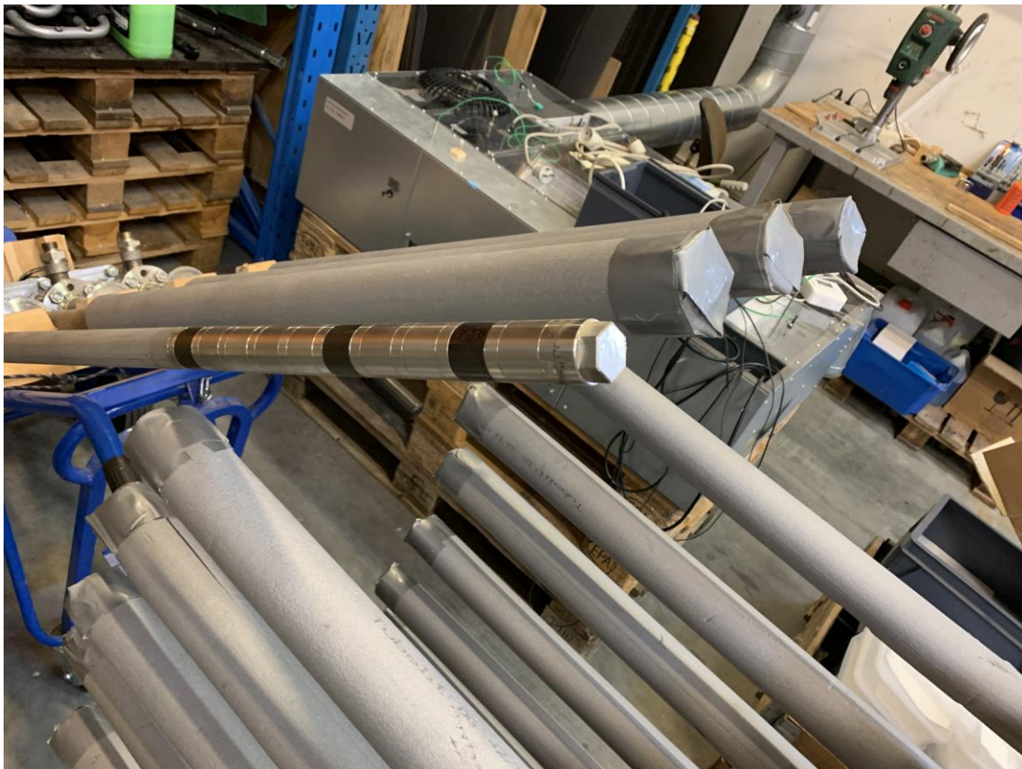
Figure 15 Probes and Coupons ready for new monitoring programmes.
