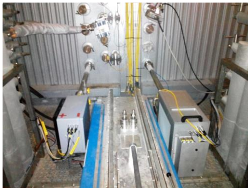
Figure 9. FTIR and UV probes with automatic extraction systems installed at AffaldPlus+ during the pilot test.
