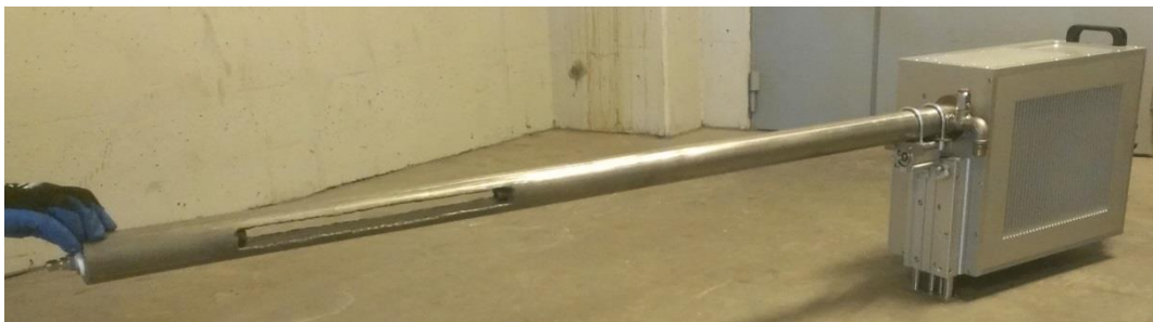
Figure 12. FTIR probe before installation. The probe is mounted with 4 screws on extraction system and can quickly be connected electrically to the control and data system.
