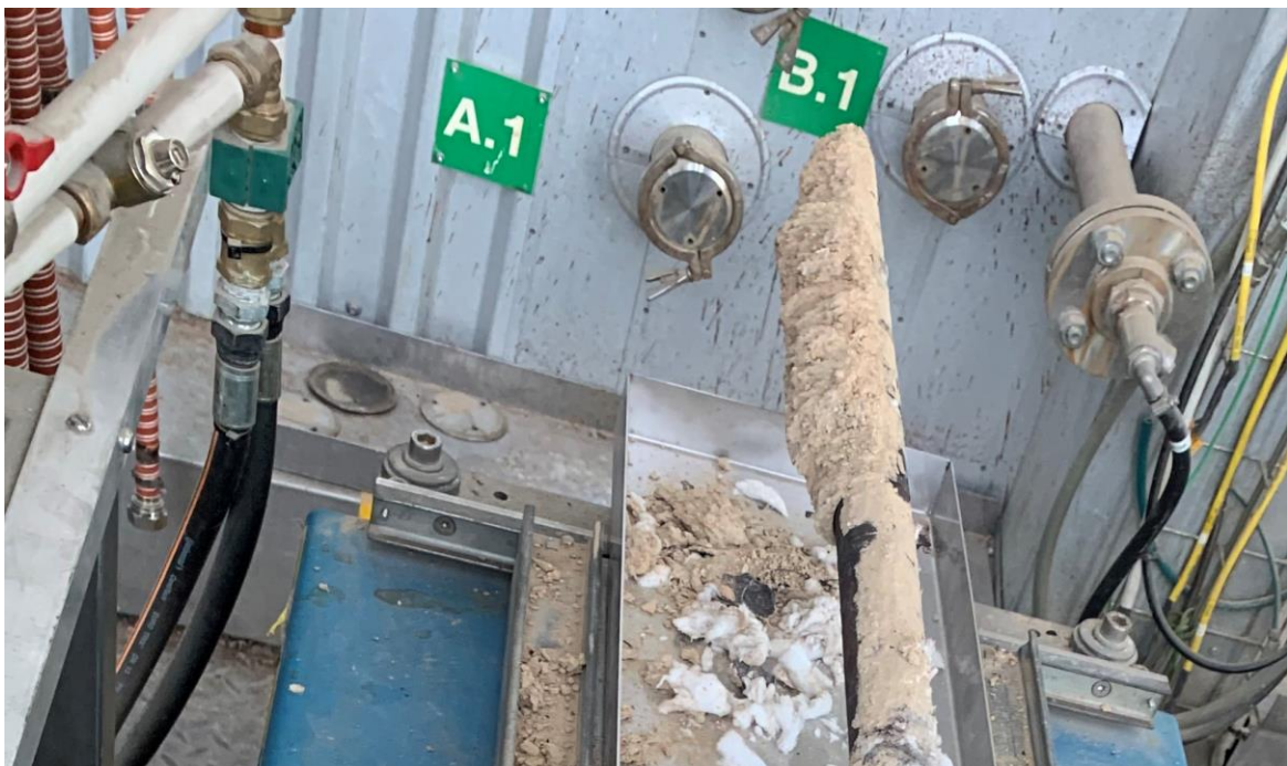
Figure 14 – Large amount of flyash on the probes – after only 6 days in operation
