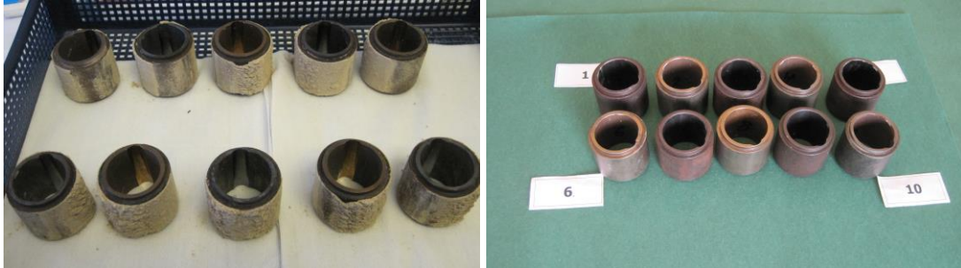
Figure 13. Ten corrosion coupons after exposure and cleaning.
