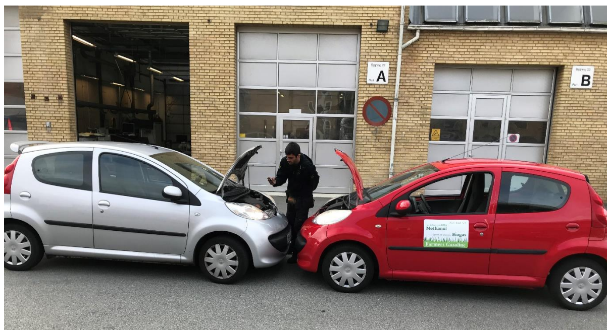
Figure 9 Sound test on two identical cars, one with gasoline (left) and one with E85 (right)
