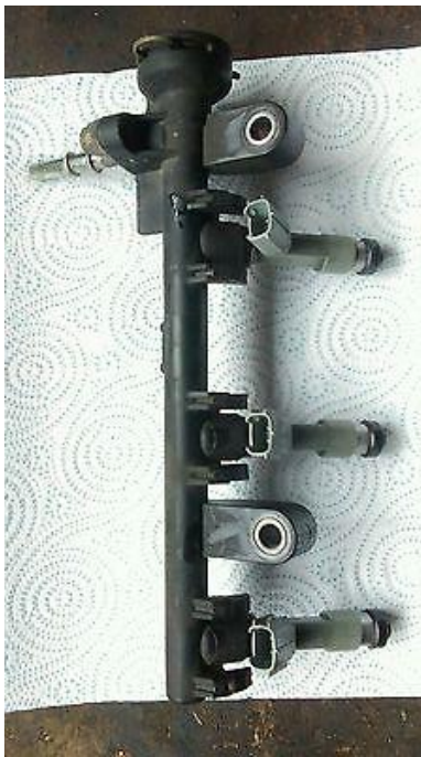
Figure 3 Fuel rail with 3 injectors (left) - Different types of connectors (right)
