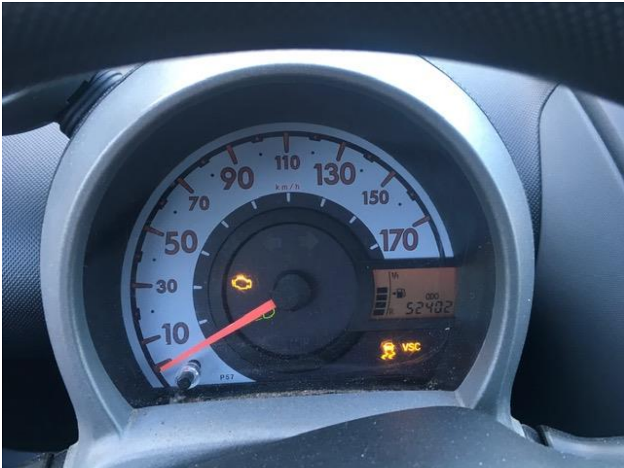
Figure 4 Max acceleration uphill can cause error. "P0171 System Too Lean Bank 1" and "P0130 O2 Sensor Circuit Bank 1 Sensor1". The errors turn on "Check Engine" light. The diagnostic trouble codes can be cleared with an OBD2 dongle.
