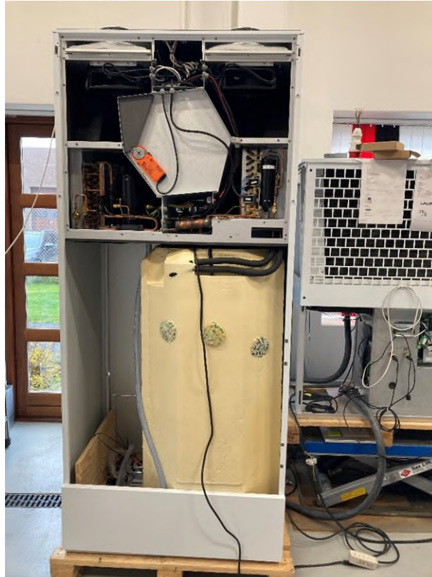
Figure 10: Prototype 2 without cover. The insulated water tank is placed in the lower part. The tank is equipped with a number of thermocouples inside the tank and at the condenser pipes wrapped around the tank as part of the DTU part of the project. The data logger for the DTU thermocouples is placed in the bottom of the cabinet, beside the water tank.
