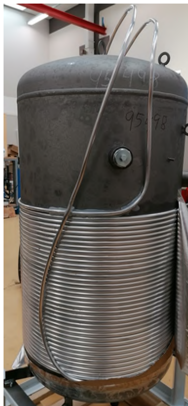
Figure 1: Experimental set up of tested tank with wrapped around heat exchanger at DTU laboratory.
