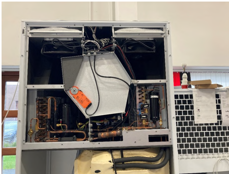
Figure 11: Prototype 2. The “refrigeration system” and the passive heat exchanger is placed in the upper part of the unit.
