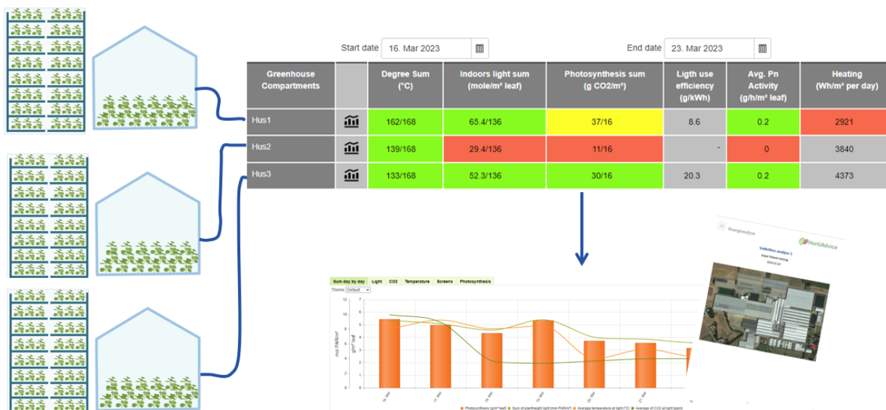
Figure 8 Data from each greenhouse are presented as rows in the summary table. The summaries are made over a period of dates that can be selected. If more detailed information's needed, charts can provide detailed data, or a detailed energy analysis can be made.
