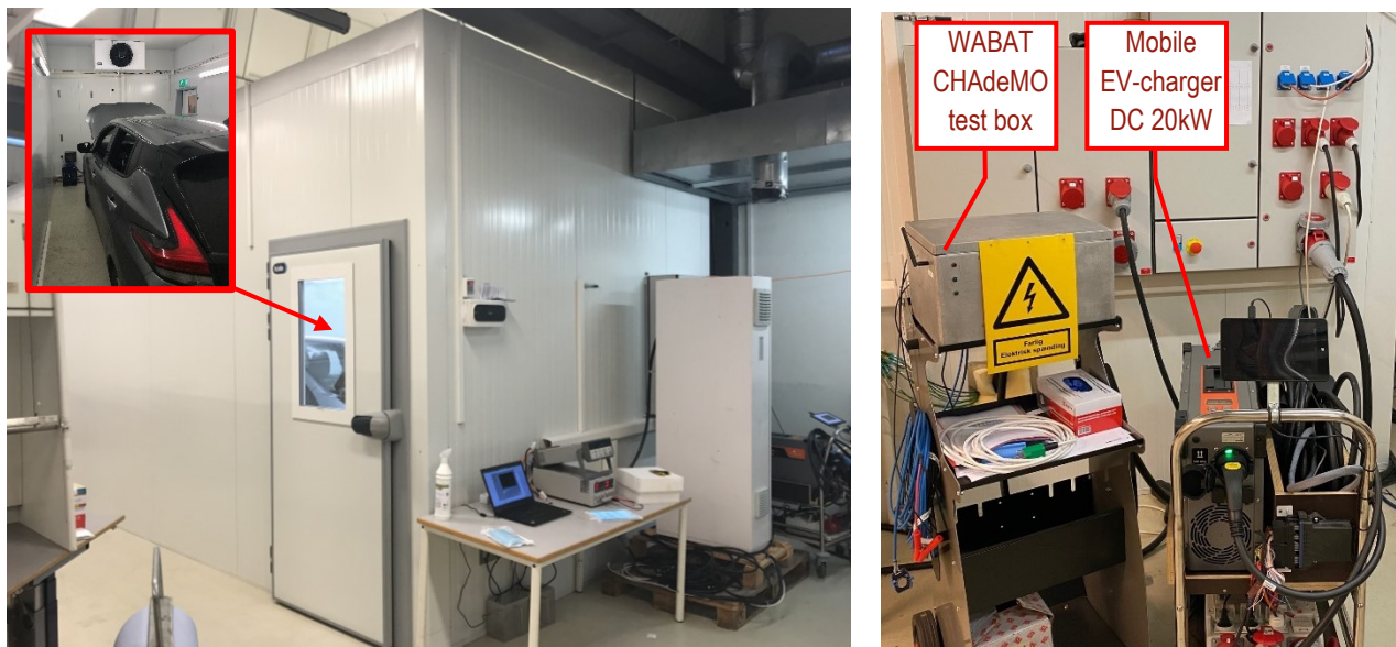
Figure 1 Temperature controlled garage for EV-test established at DTI specifically for performing WABAT EV test under consistent conditions. The tall cabinet at the end of the garage is a CHAdeMO V2G charger 10kW on temporary loan from NUVVE. The vehicle in the garage is a Nissan Leaf 62kWh, that has been tested at regular intervals throughout the project period. In the right picture the WABAT CHAdeMO box is used for test.
