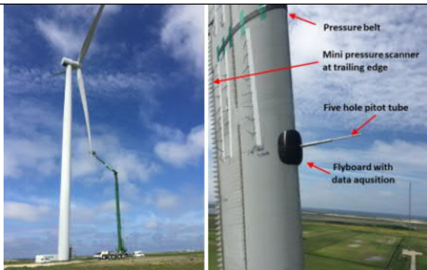
Figure 7. Overview of the pressure belt and inflow sensor being tested in full-scale in June 2021.
