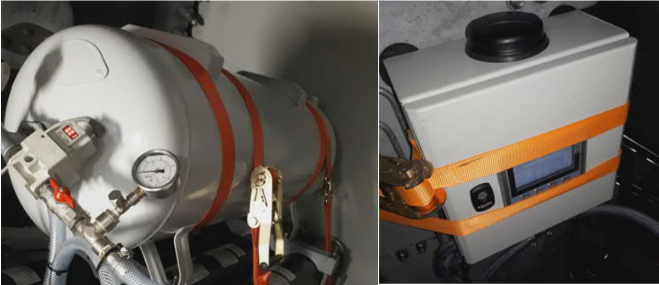
Figure 5. Third generation of pressure supply system and control box.
