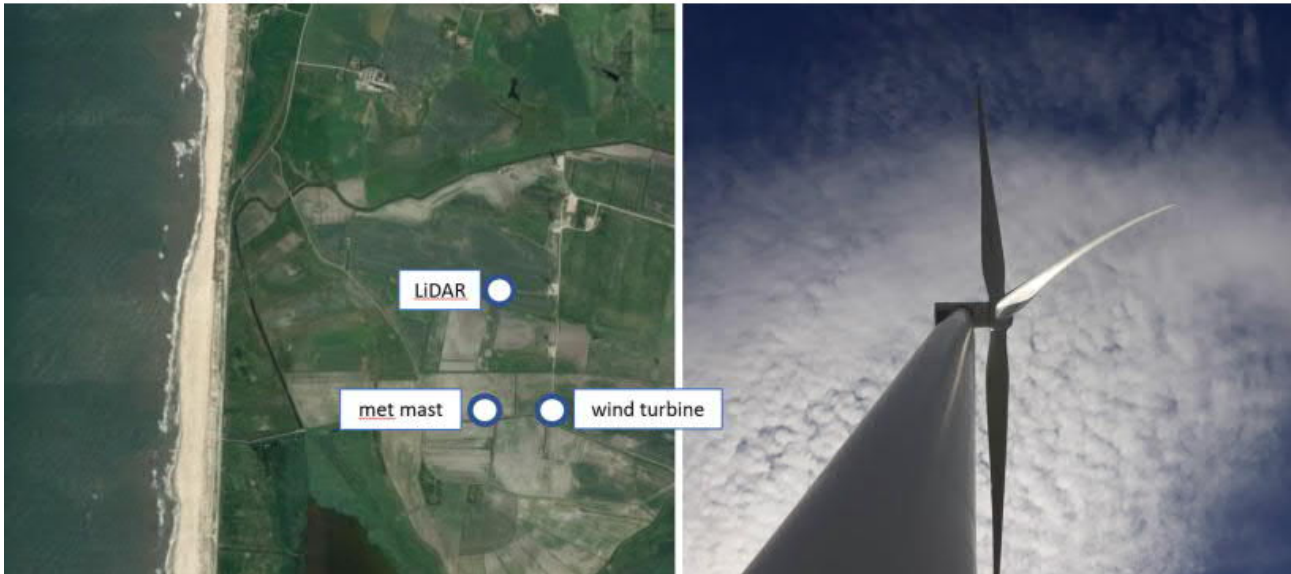
Figure 9. SG 4.3-120 DD turbine used for full-scale characterization of the active flap system in the test site Høvsøre.
