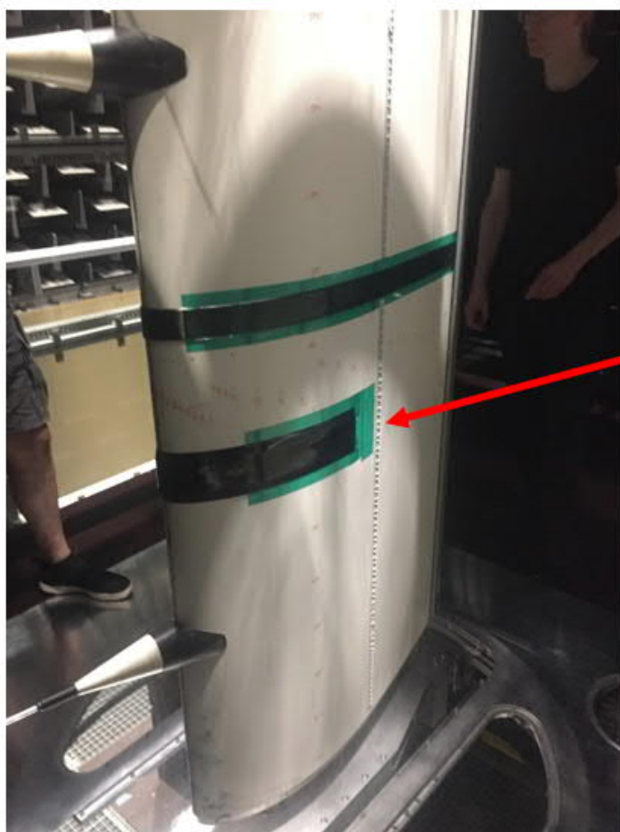
Figure 2. View of the pressure belt being tested in the wind tunnel.
