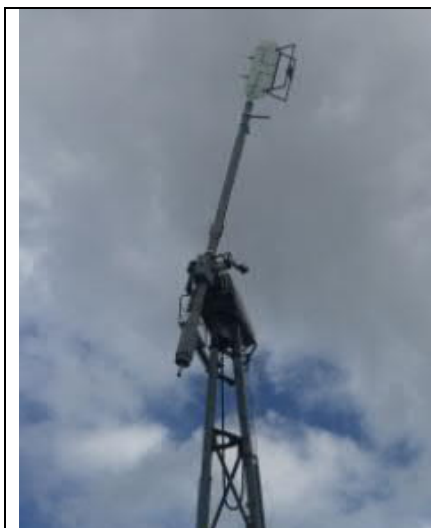
Figure 6. The wake rake developed within the INDUFLAP2 project for measurements of the drag on a rotating blade section. Here the rake is attached on a 2.0m blade section mounted on the rotating test rig at the Risø Campus at DTU.
