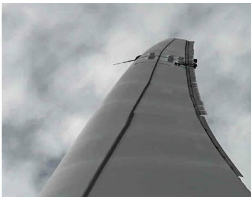
Figure 8. View of the active flap system during characterization tests of instrumentation systems
