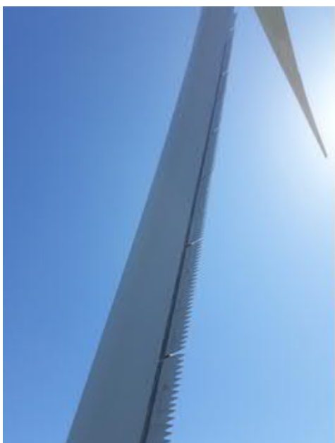
Figure 8. View of the active flap system during characterization tests of instrumentation systems
