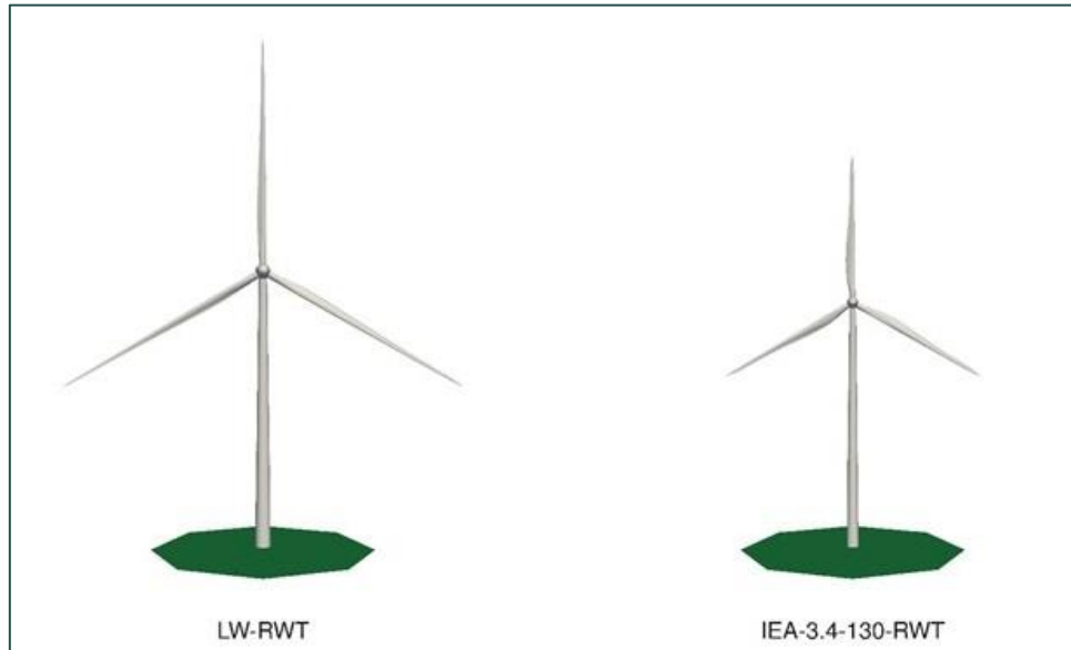
Figure 1 To the right the conventional turbine with a rotor diameter of 130 m which gives a specific power (SP) of 256 W/m 2 based on the rated electrical power of 3.37MW. To the right the 208m diameter LowWind reference wind turbine (LW-RWT) designed and developed in the present project with specific power of 100W/m 2
