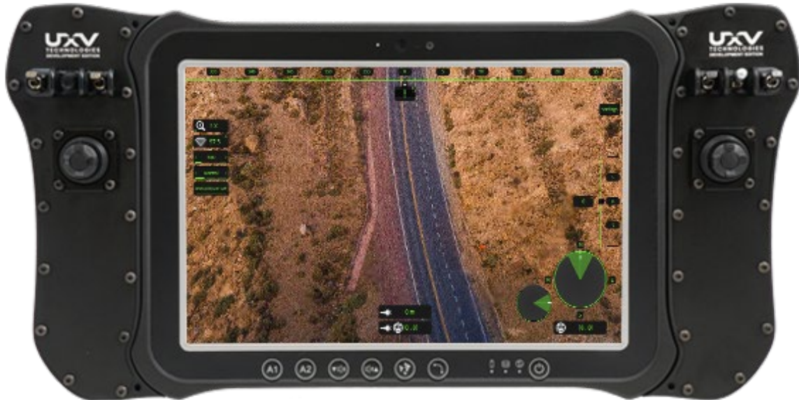
Figure 5.1.2 Gimbal controller which will be tailored to control the DronEL payload.
