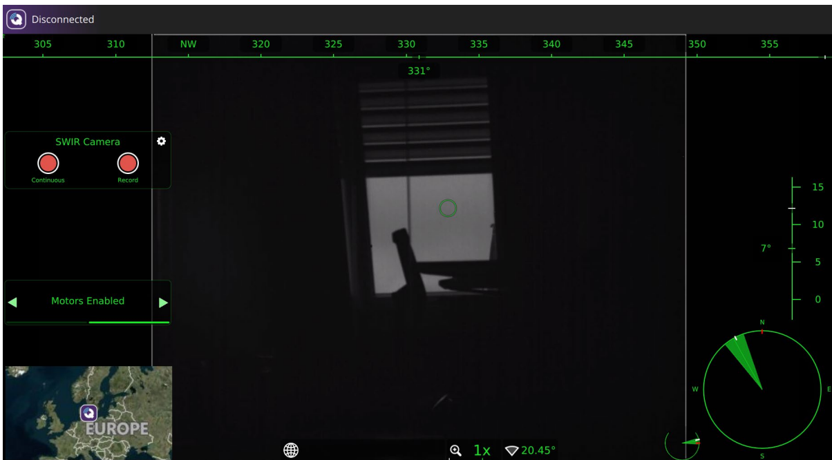
Figure 5.5.3 QGround Control APP graphical user interface for live video streaming and control of the drone payload.
