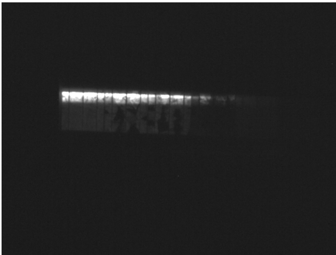
Figure 5.5.2 - Image frame of the laser scanning a PV module. Three cells are covered by the laser's high power region.
