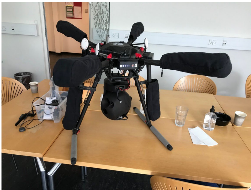
Figure 5.3.2 – Photos of the developed DronEL payload.
