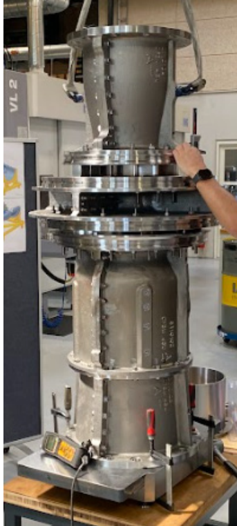
Figure 5 Expander / Compressor at mounting
