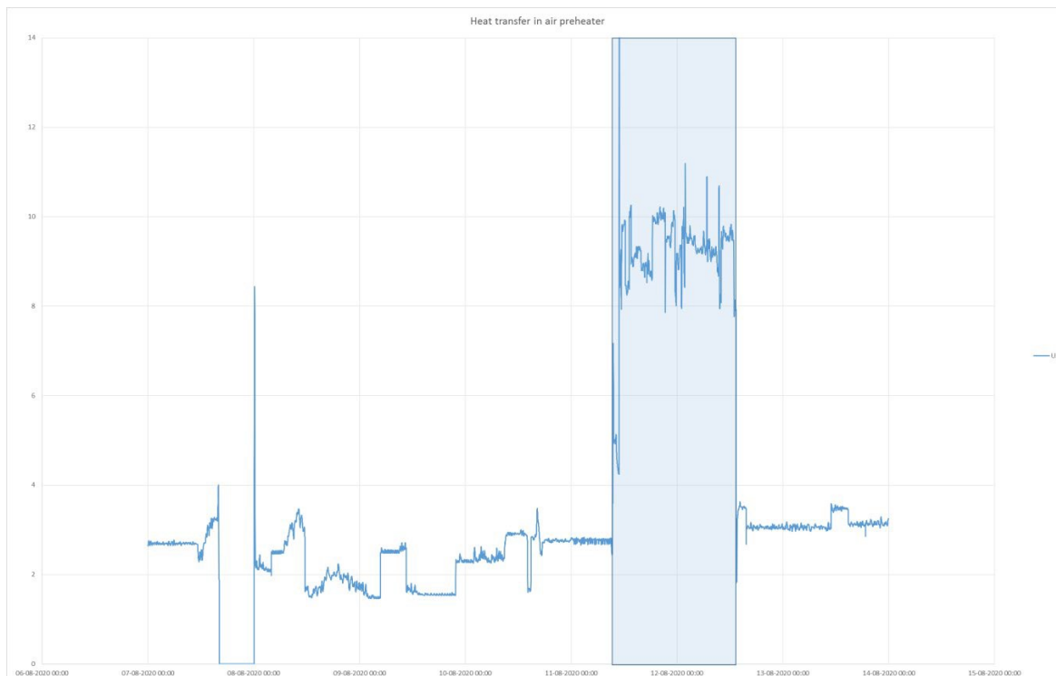
Figure 6 Overall heat transfer for the air preheater. Marked area indicates period where the test was executed.
