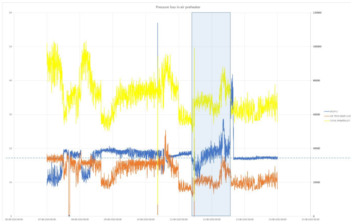
Figure 5 Pressure loss over air preheater compared to flow and squared flow. Marked area indicates period where the test was executed.
