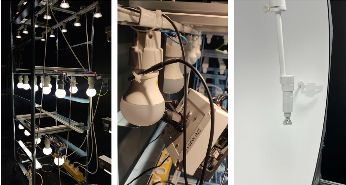
Figure 18 – Endurance testing of LED lamps and modules. The devices are operated in standardized conditions for several thousands of hours. A monitor system logs the intensity and temperature over 5-8 months. At regular intervals, the light output is measured in the integrating sphere. The project has compared the new EU on/off cycling endurance test with continuous on lifetime test. Photos: DTU Electro.
