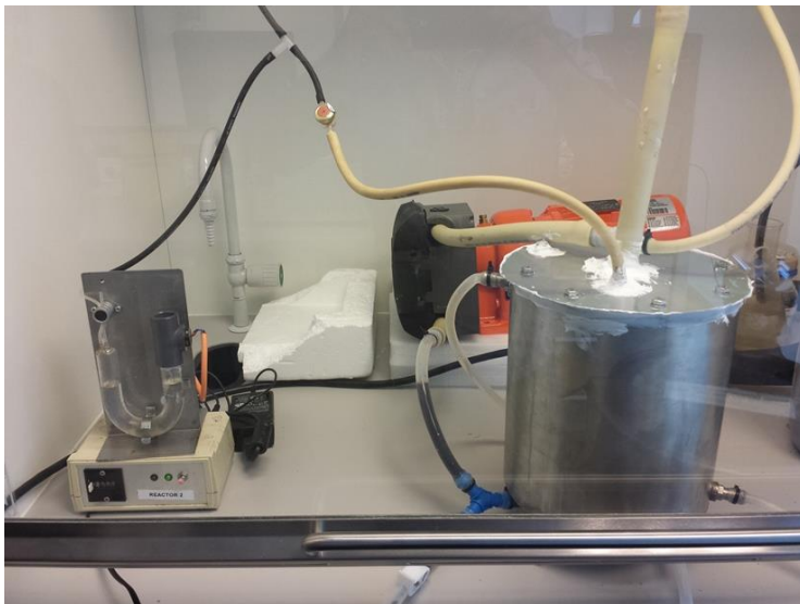
Figure 2.2. Lab-scale single stage reactor of OFMSW involving percolating and recirculation
