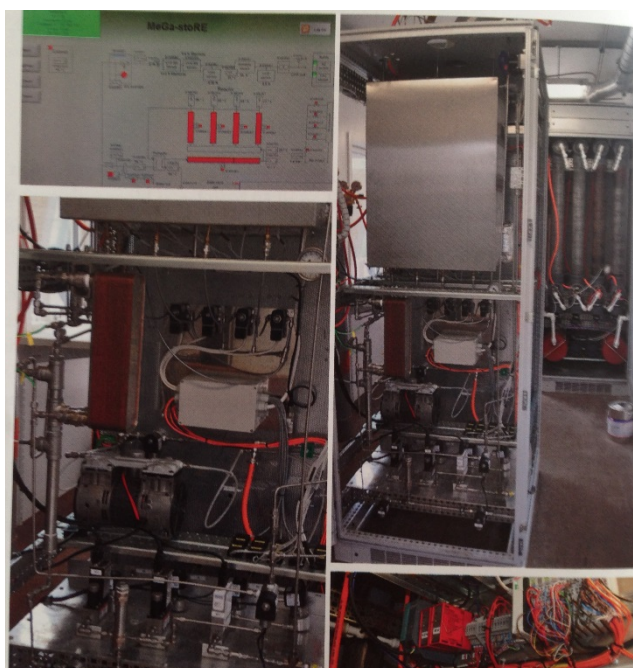
Figure 1 MeGa-stoRE, proof-of-concept plant. Consisting of a cleaning unit and a methanation plant with computer controlled process regulation with comprehensive data collection from both units.
