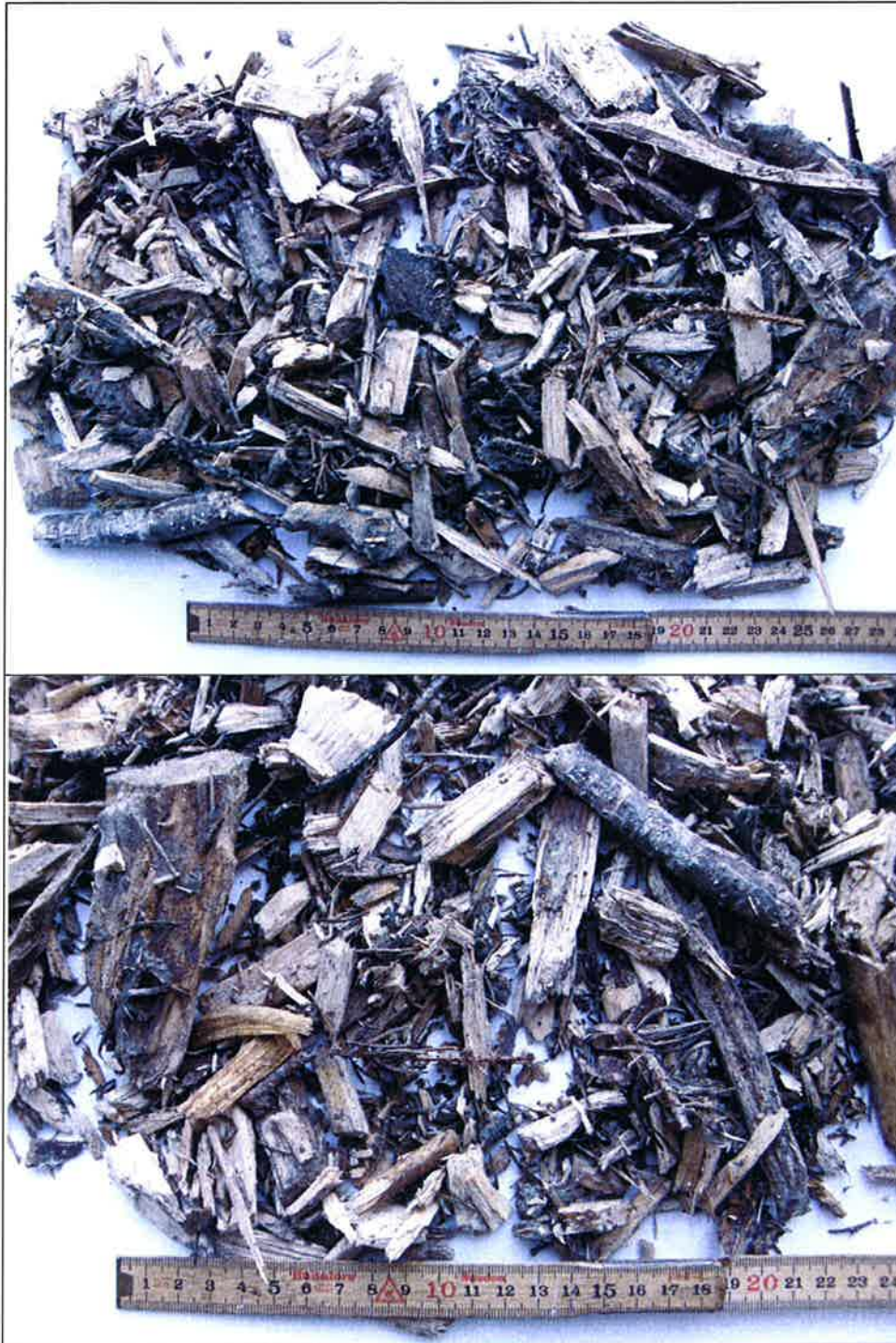
Figure 6. Pictures showing the fresh wood chips burned in the furnace
