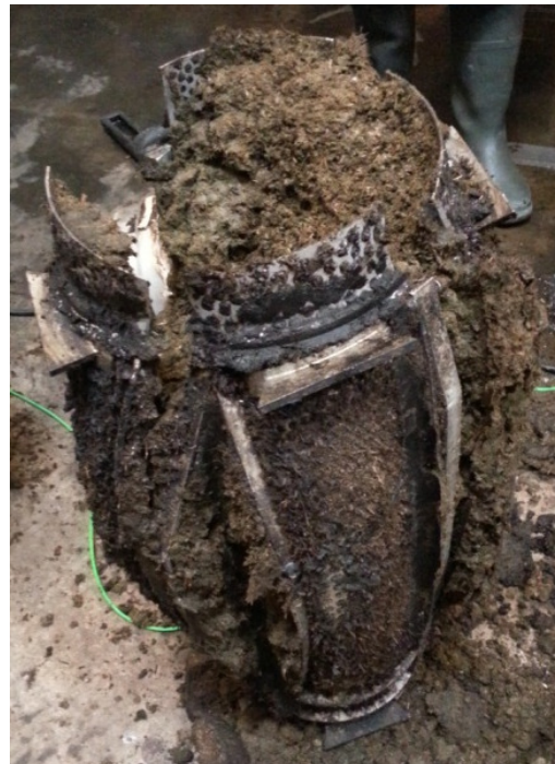
Figure 11. The ruptured sieve caused by feeding biomass to the dewatering unit after the dewatering stopped running.
