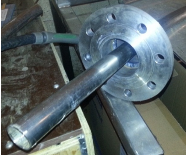
Figure 13. The elongated flash-out pipe. The pipe goes through the compensator which is bolted to the flange.
