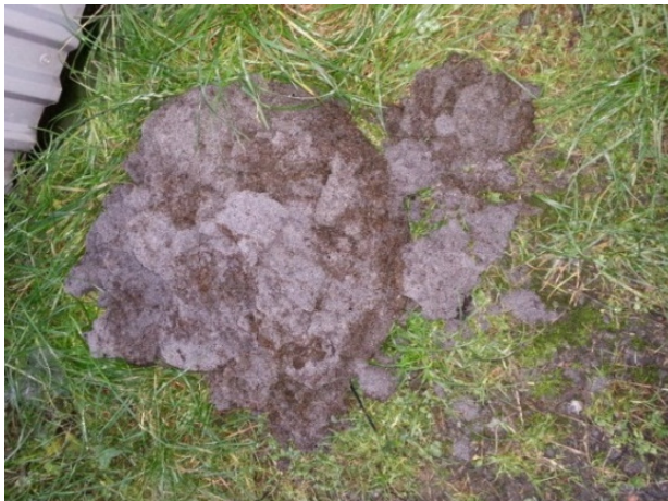
Figure 14. A portion of the sand removed from the monotube heat-exchanger after a blocking.
