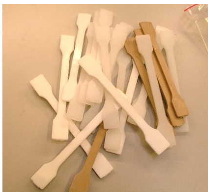
Figure 3: 'Dog bone' samples for tensile test
