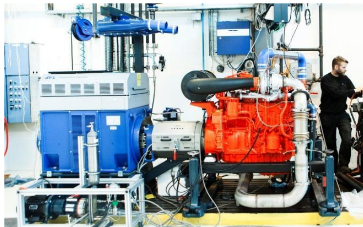
Figure 8: Scania engine coupled to the dynamometer at TI-Engines
