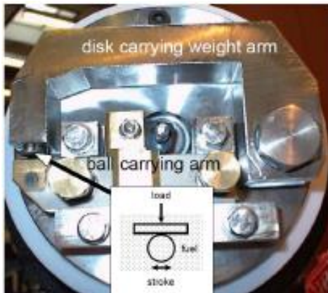
Figure 13. MPFRR test setup at DTU
