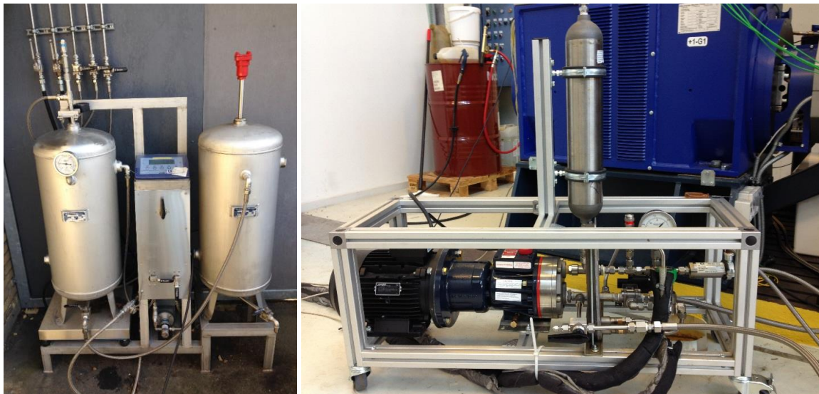
Figure 10: Fuel mixing station (left) and the boost pump rig (right)
