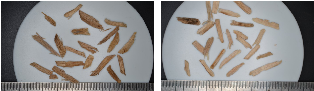
Figure 13. Comparison of large particles: Left=30%moisture, Right=5%moisture
