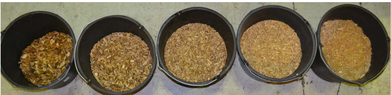
Figure 11. Picture of chopped wood chips at different speeds. From the left to the right: 30 m/s, 65 m/s, 100 m/s, 145 m/s and 200 m/s
