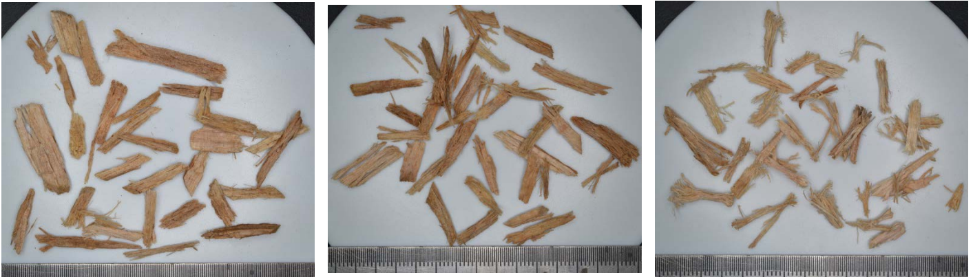
Figure 14. Picture of fraction > 3.15 mm after 1, 2 and 3 passages through the chipper
