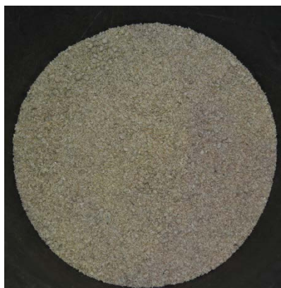
Figure 15. Picture of downsized wood pellets at 100 m/s
