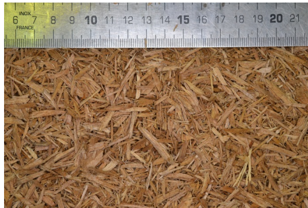
Figure 12. Wood chips downsized at 200 m/s
