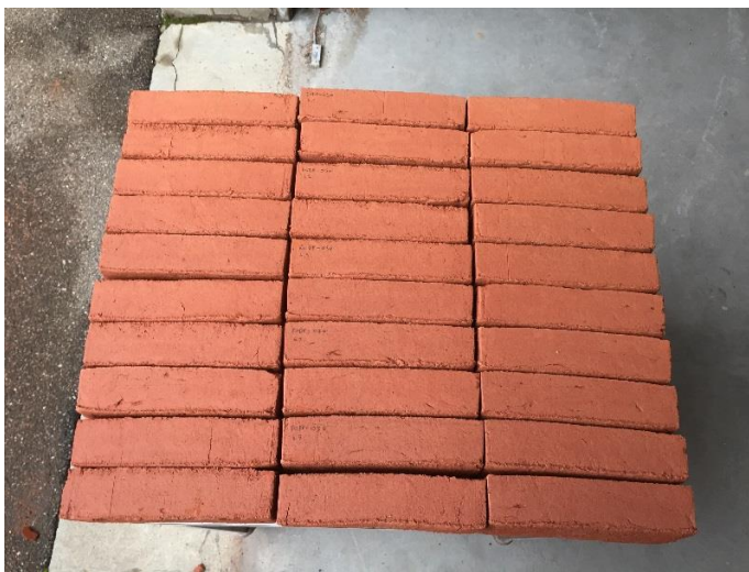
Fig. 7b: Optimized MAGF firing, uniform colour
