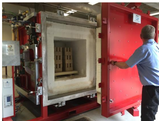
Fig. 5b: First test run in Aarhus after delivery. The kiln is equipped with 4 gas burners and 2 microwave generators, each with 2 ports. The power supplies for MW generators are water-cooled.
