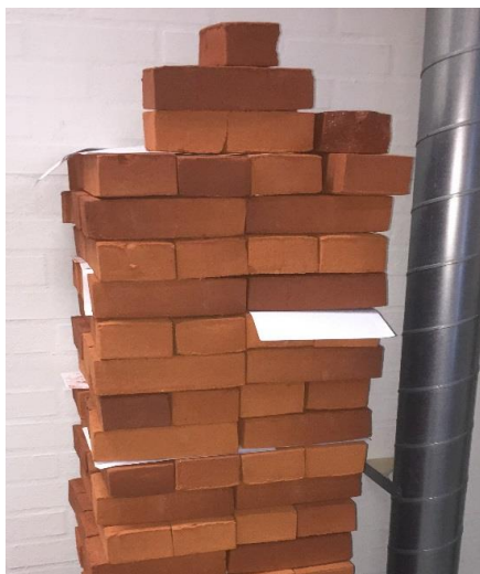
Fig. 7a: Early gas firing with dense load and resulting colour variations
