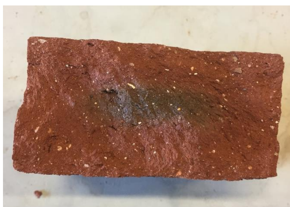
Fig. 6b. Reduction core in the centre of stone fired with gas, with rapid heating.
