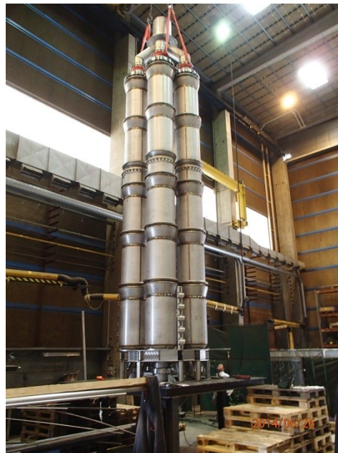
Test assembled reactor internals
