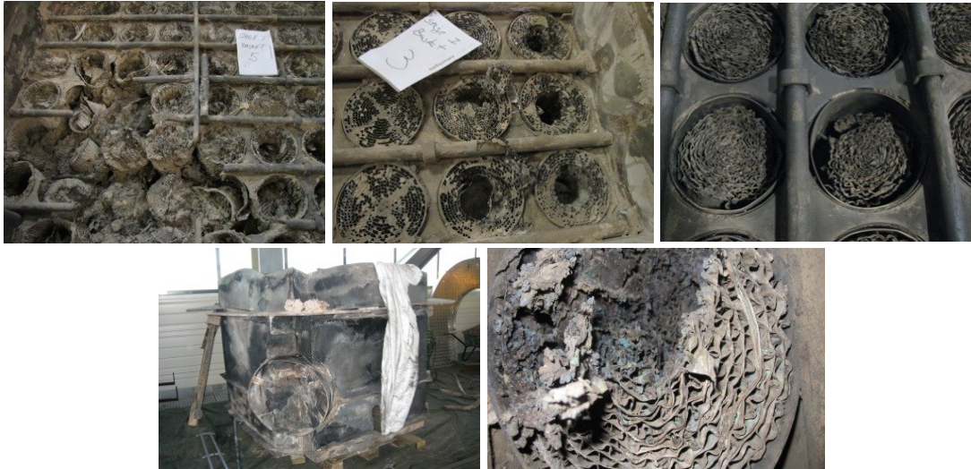
Picture 2 Damaged and partly melted trays
