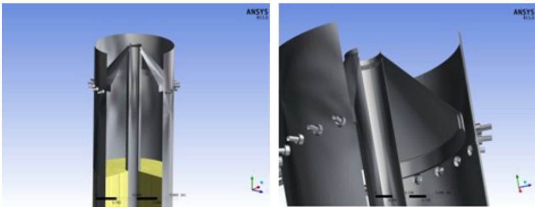
Picture 4 Geometry of MEGA monolith installation used in CFD simulation of reactor internal
