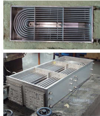
Fig. 4.23. Storage system installed in the pilot plant.
