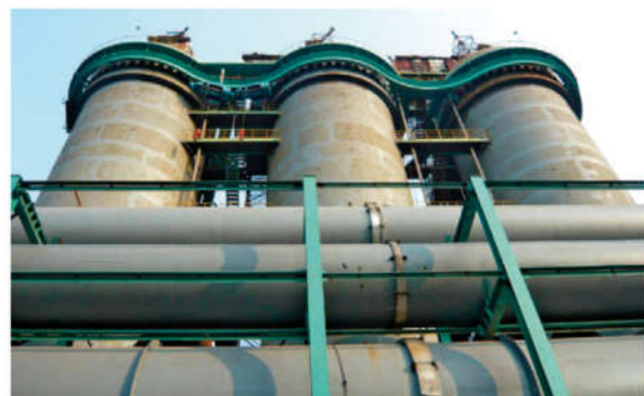
Fig. 4.5. Cowper stoves at Hyundai Steel Corporation (L) and Zhangjiagang Pros Iron Making (R) [42].
