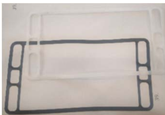
Fig. 12 Teflon gasket (white) and FKM gasket (black).
