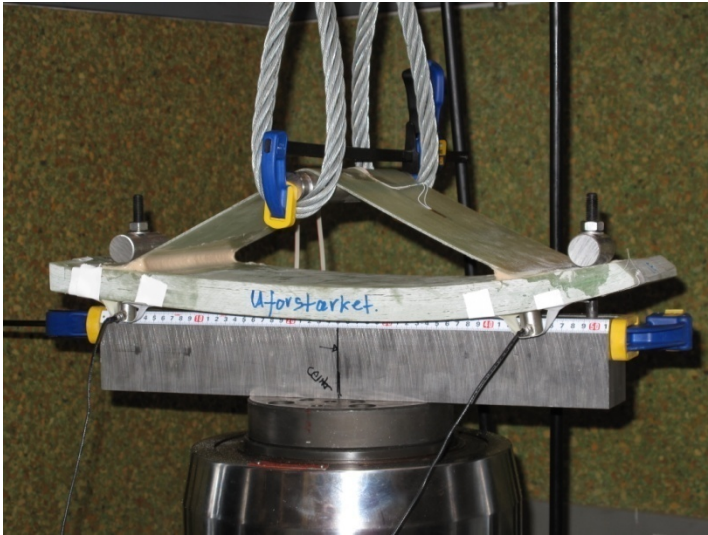
Figure 45: Test setup for measuring the load capability of the transverse reinforcement.
