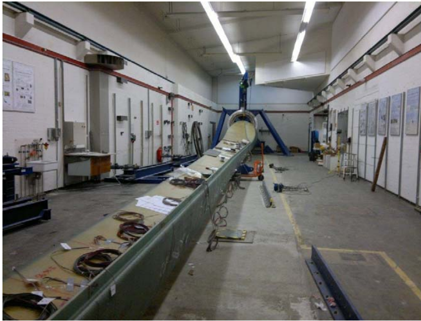
The DMT Box Beam under preparation in the test hall prior to being mounted on the test rig
