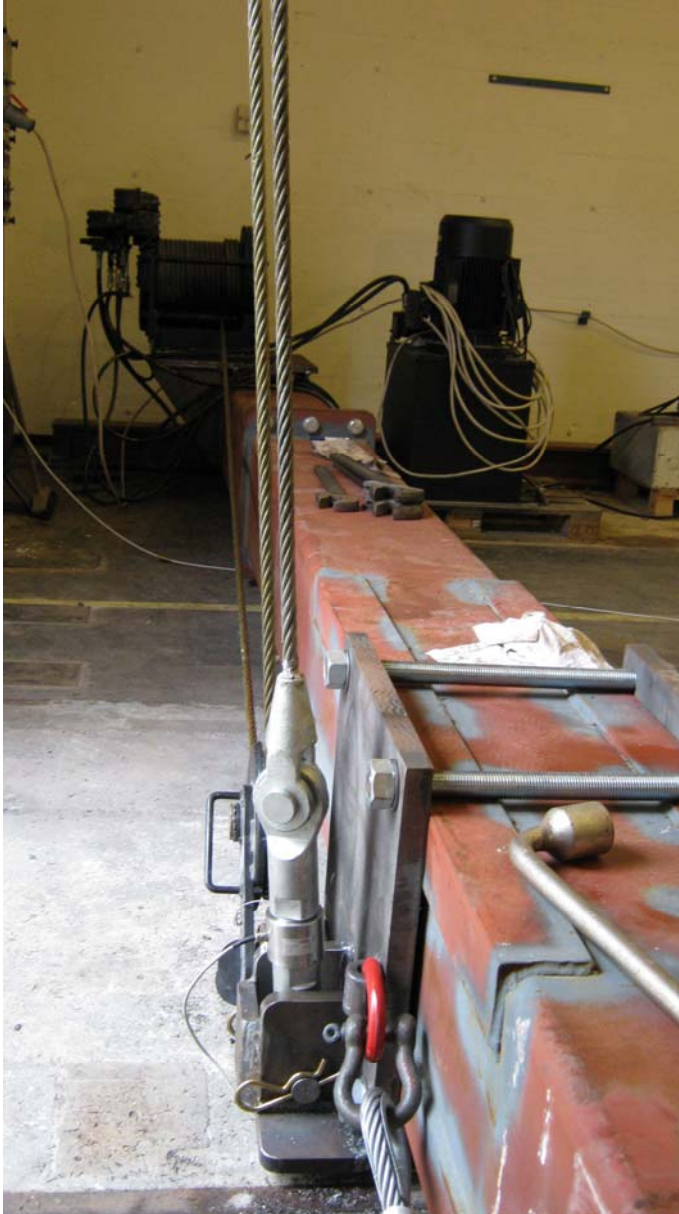
Figure 59: A photo of the steel girder for applying the load. In the back the winch is shown, and in the front, the bracket for guiding the wire to the girder is shown.
