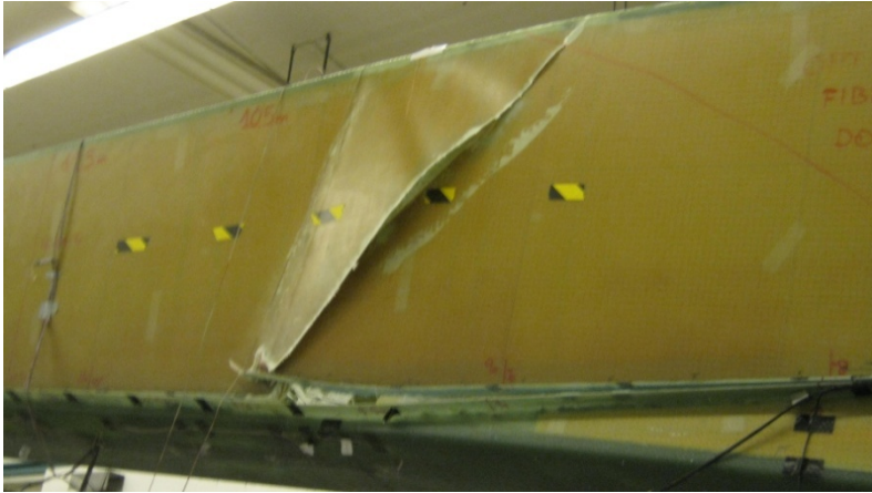
Figure 82 Photos showing damage on the web at around 10m section
