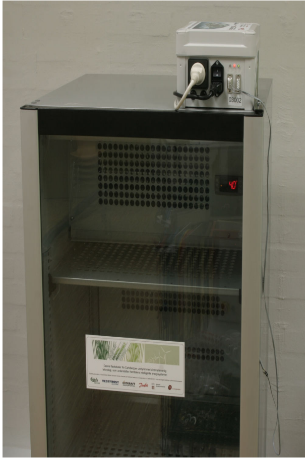
Figure 4. DFRC device placed on the top of refrigerator, with serial communication wire visible.
