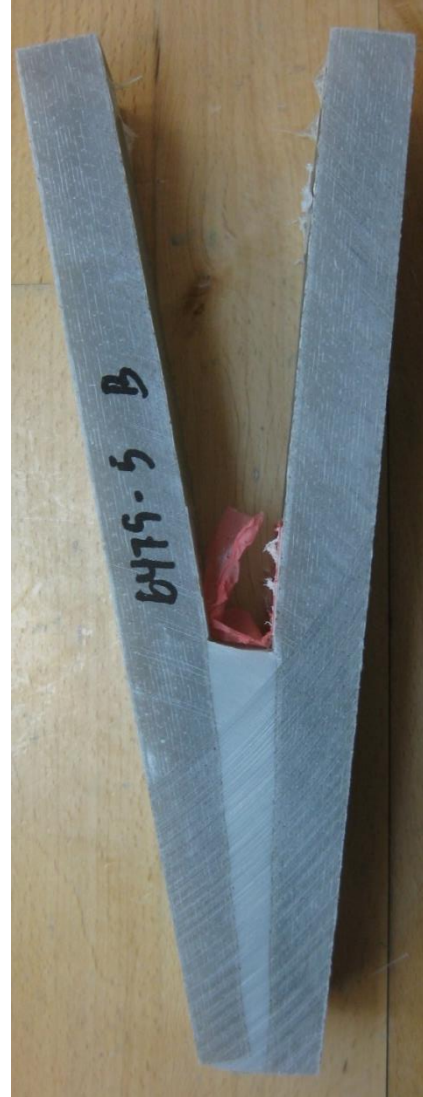
Figure 79: Specimen of the series h2/t2 , \alpha = 15^\circ , t = 15\text{mm} , h = 20\text{mm}
