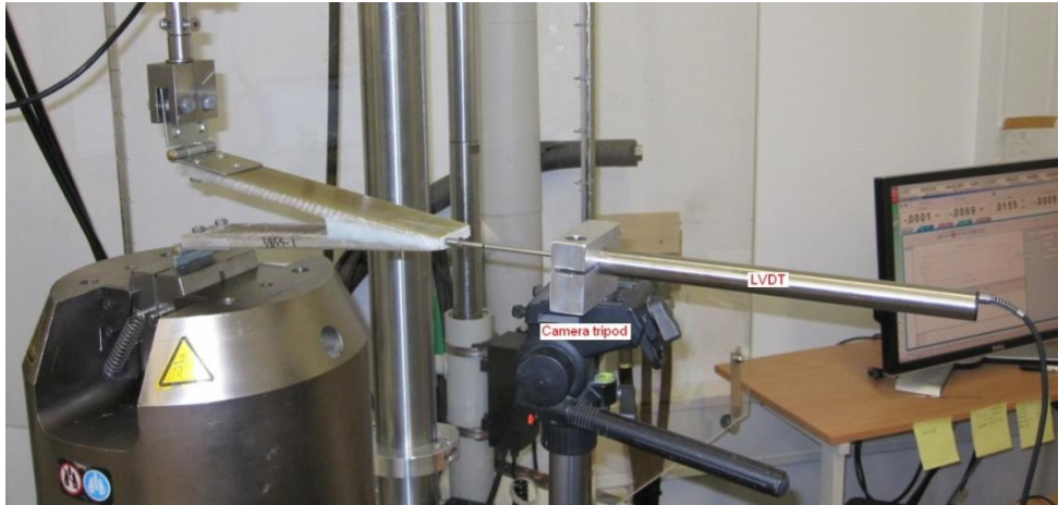
Figure 98: Test setup with LVDT and camera
