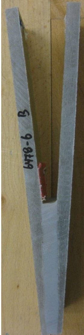
Figure 77: Specimen of the series h1/t1 , \alpha = 10^\circ , t = 10\text{mm} , h = 10\text{mm}
