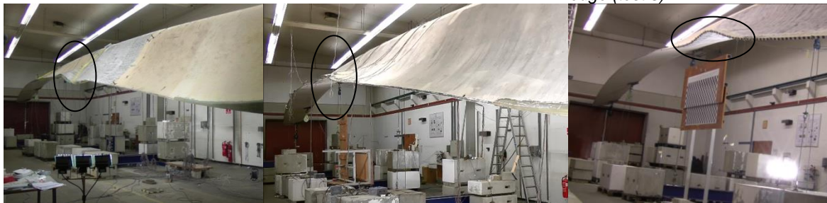
At approximately 55% load, ultimate failure (test 1)
