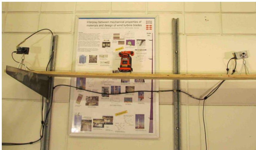
Figure 21 Two cameras on tripods sitting on a shelf at an elevated height facing the trailing edge. The wires seen are part of the electronic shutter system enabling simultaneous triggering of digital cameras. Laser level (red) used to adjust the calibration grid alignment.
