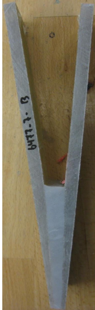
Figure 78: Specimen of the series h1/t2 , \alpha = 15^\circ , t = 15\text{mm} , h = 10\text{mm}
