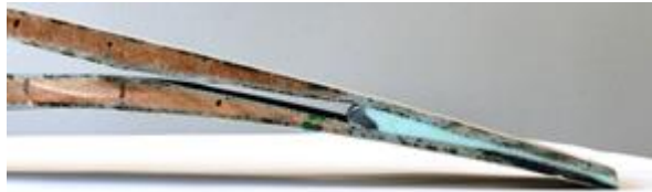
Figure 36 Detail of trailing edge joint showing the bonded area with laminate and the panels with sandwich core material where sensors in the sandwich core area gave a noisier signal when compared to sensors placed within the pure laminate.
