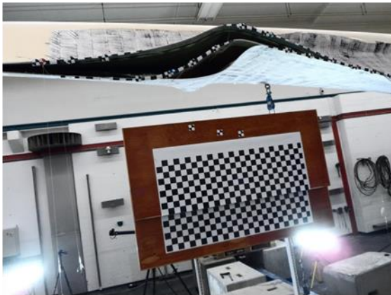
Figure 30 Trailing edge deformation at different load level for the multi-point loading test. (top left) prior to loading, (top right) 40% of load and (bottom) ultimate failure due to local buckling induced debonding of the trailing edge joint. (partially taken from Haselbach et al. (2015))
