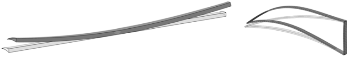
Figure 60 (left) 3D shell model of main beam with superimposed deformation plot; (right) cross-section beam slice taken from mid span with superimposed cross-section deformation. Deformation scale factor 10. (taken from Eder & Bitsche (2015))
