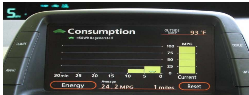
Figure 8: Descriptive dashboards provide instant feedback to drivers in order to effect better driving habits.
