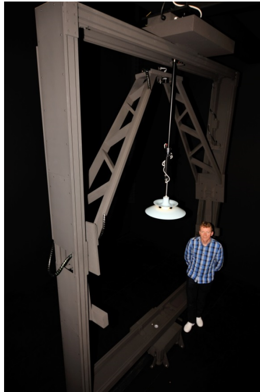
Figure 38. Top: 2m integrating sphere used to measure the total spectral flux of luminaires. Right: Goniophotometer used to measure the light intensity distribution of the luminaires.
