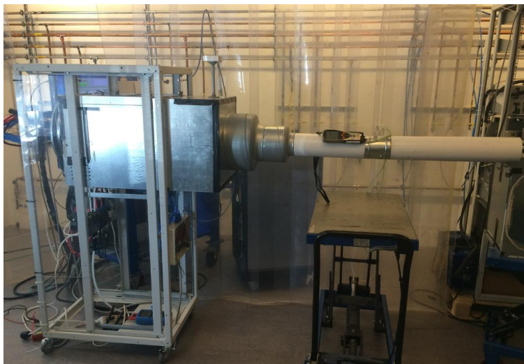
Figure 24: Picture from the bypass testing performed on the 3rd generation climate kit at Cemtec
