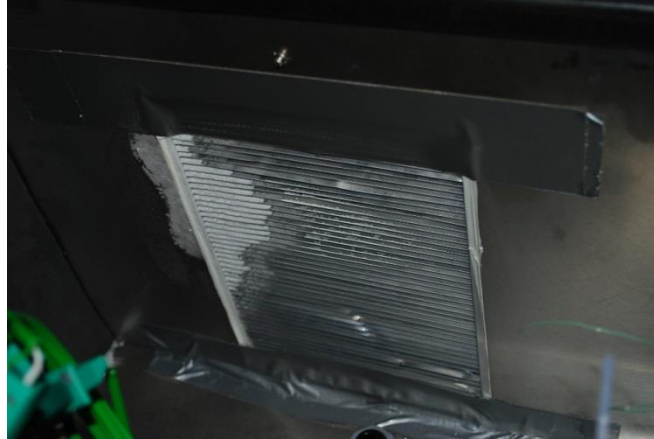
Figure 15: Both cross and counter flow heat exchangers turned out to have icing problems because of the water content in the cathode exhaust stream.
