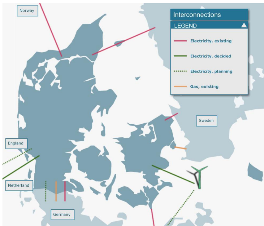
Figure 16. Existing (in red), decided (in green) and planned (in dashed green) Danish interconnections to neighbouring countries, as per September 2015 (Energinet.dk, 2015).
