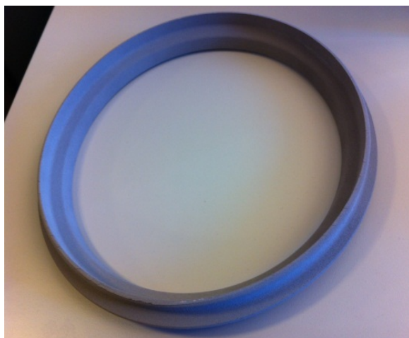
Figure 41: Printed and sintered Ni40Cr3.5Nb material for use in the seat area of the valve spindle.
