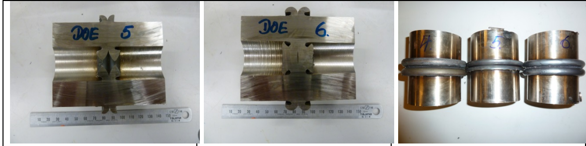
Figure 30: Welding flash geometry on a selection of samples
